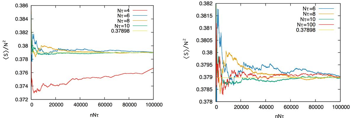
Figure 14:  $\langle S \rangle / N^2 = \frac{1}{n} \sum_{k=1}^n S[\phi^{(k)}]$  with  $N = 100$ , for several different values of  $N_\tau$ . The horizontal axis is  $n \times N_\tau$ , which is proportional to the cost (time and electricity needed for the simulation). We can see that  $N_\tau = 8, 10$  are more cost effective; i.e. better convergence with less cost. Note that we started the measurement runs with well thermalized configurations.
