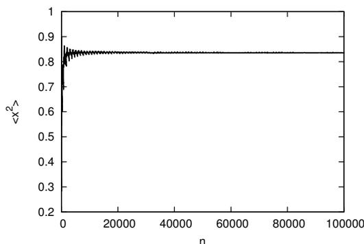
Figure 12: Gaussian integral with Metropolis,  $c = 1$ , with *non-random* numbers; we chose the same random number sequence every 1000 steps.  $\langle x^2 \rangle = \frac{1}{n} \sum_{k=1}^n (x^{(k)})^2$  converges to a wrong number, which is different from 1.
