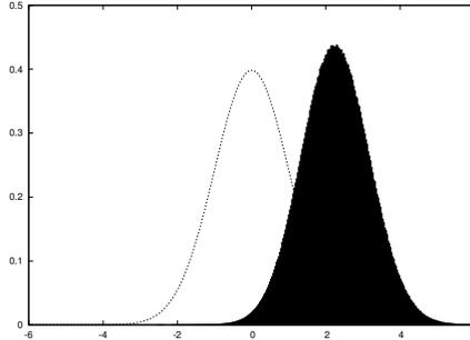
Figure 4: The distribution of  $x^{(1)}, x^{(2)}, \dots, x^{(n)}$  for  $n = 10^7$ , with *wrong* algorithm with  $\Delta x \in [-\frac{1}{2}, 1]$ . The dotted line is the right Gaussian distribution  $\frac{e^{-x^2/2}}{\sqrt{2\pi}}$ .
