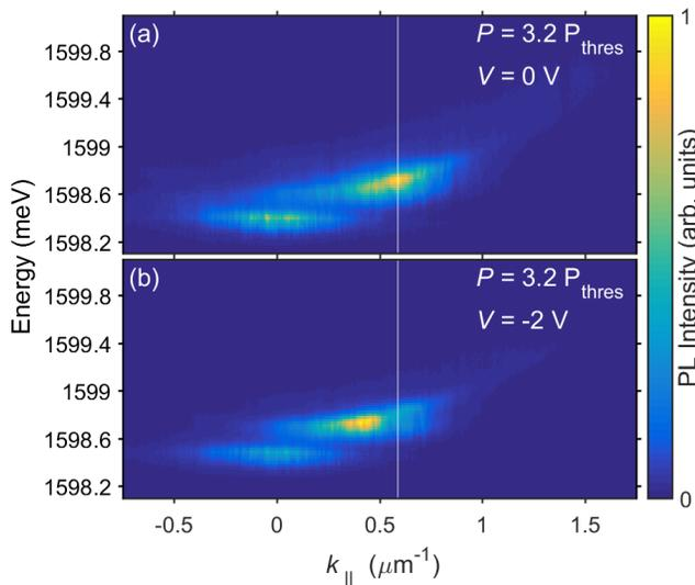
FIG. 3. PL intensity vs. energy and in-plane momentum ( $k_{\parallel}$ ). The threshold power ( $P_{\text{thres}}$ ) was about 114 mW, and the powers used were both about  $3.2P_{\text{thres}}$ . The applied voltage in each case (a) 0 V and (b) -2 V. The white vertical line is marking the  $k_{\parallel}$  value of the peak of the distribution at zero applied voltage to aid in comparing the two images. The PL intensity was normalized separately for each image.
