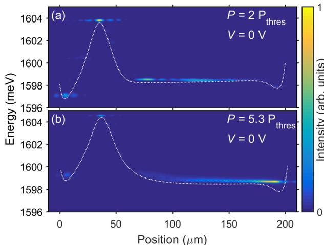
FIG. 2. PL intensity vs. energy and position along the length of the wire at zero applied voltage. The white dotted lines give the outline of the potential felt by the polaritons. The threshold power ( $P_{\text{thres}}$ ) was about 114 mW, and the powers used were (a)  $2P_{\text{thres}}$  and (b)  $5.3P_{\text{thres}}$ . The PL intensity was normalized separately for each image.
