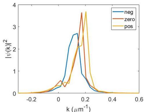
FIG. 7. Time-integrated average momentum of the polaritons in the condensate corresponding to the theory plots in Figure 6.
