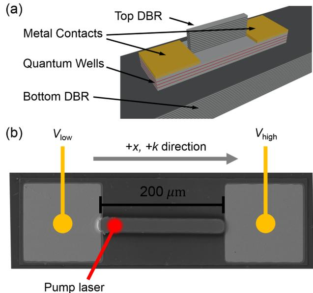
FIG. 1. a) The etched microcavity structure with the NiAuGe contacts at each end of the wire. (b) Scanning electron microscope (SEM) image of a representative etched wire, with an overlay showing the experimental arrangement. The voltage connections of the source were connected to the device as shown. Thus, positive conventional current flowed in the direction of  $-x$ .
