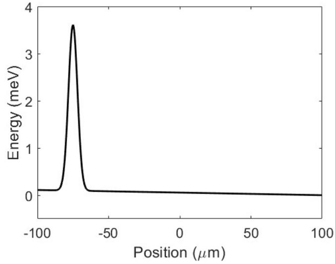
FIG. S4. Effective potential  $V_\psi$  experienced by the polaritons in the wire in the simulations. The ends of the wire are modeled as an open boundary condition.
