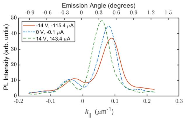
FIG. 4. Time integrated average momentum distribution of the condensate under different applied voltages for the wire shown in Fig. 5. These data are for a wire similar to that used for Figure 3, but with a smaller cavity gradient  $0.0025 \text{ meV}/\mu\text{m}$  and a smaller threshold power of  $P_{\text{thres}} \approx 75 \text{ mW}$ . The power used was  $10.3P_{\text{thres}}$ .
