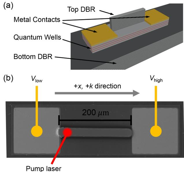
FIG. 2. (a) The etched microcavity structure with the Ni-AuGe contacts at each end of the wire. (b) Scanning electron microscope (SEM) image of a representative etched wire, with an overlay showing the experimental arrangement. The voltage connections of the source were connected to the device as shown. Thus, positive conventional current flowed in the direction of  $-x$ .
