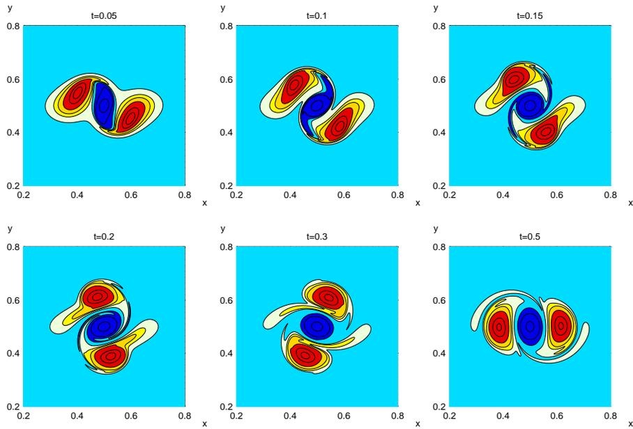
Figure 21. Tri-polar vortex (2.7) in rotation with marked shear patterns over time. Plotted iso-vorticity contours are  $-200, -150, -50, 1, 5, 20, 40, 55$  and  $\pm 10$ .
