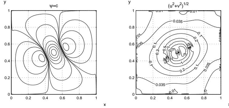
Figure 20. Stream function and velocity at  $t = 0.25$  of the preceding plot. They may facilitate the interpretation of visualisation in laboratory conditions (cf. p.15 of Samimy *et al.* 2004).
