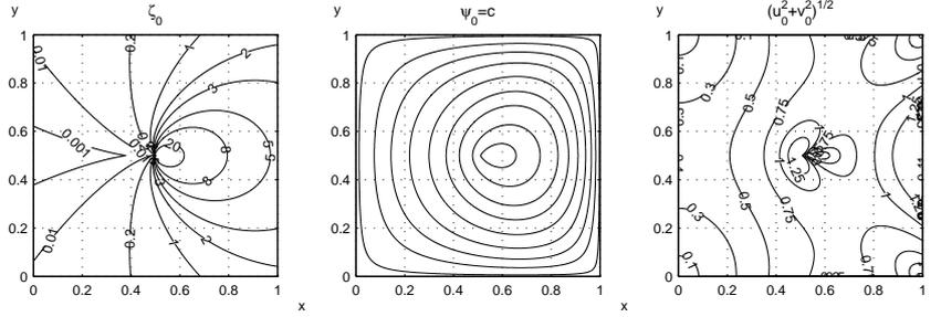
Figure 1. Isolated vortex. The data induce noticeable velocities. As soon as the motion is initiated, see figure 8, wall layers are generated and the velocities are strongly modified by viscosity so that the no-slip is fully observed.
