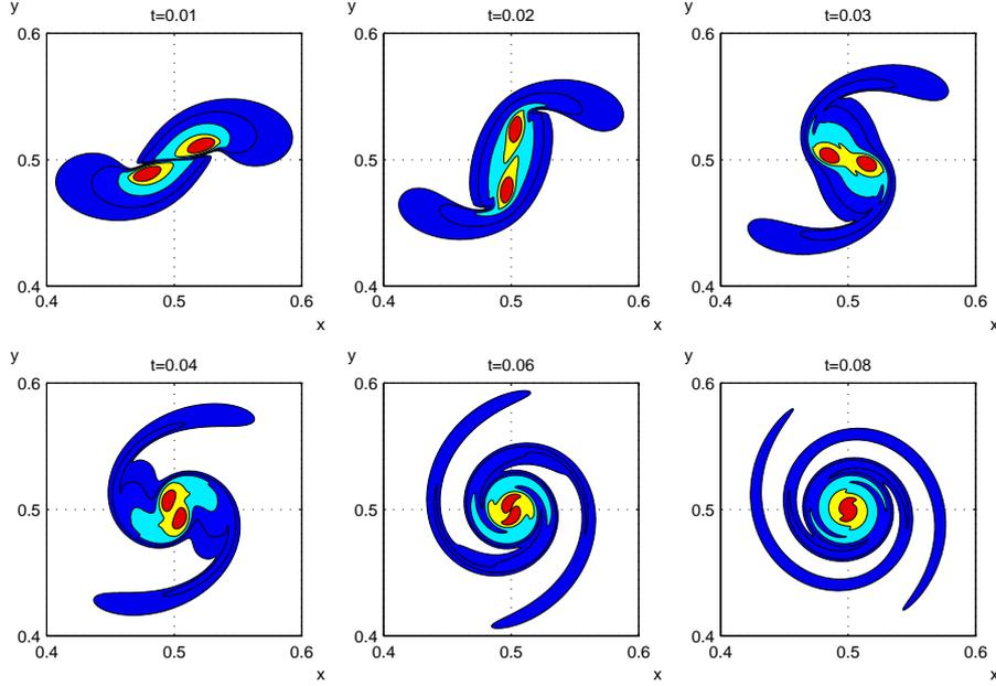
Figure 14. Zoom-in appearance shows how an S-shaped core has been born out of the revolving eyes during the initial stages of evolution. The outer fan structures are evidently dependent on the core strength and the properties of the fluid. Iso-contour levels are 50, 100, 200, 400 and 600.
