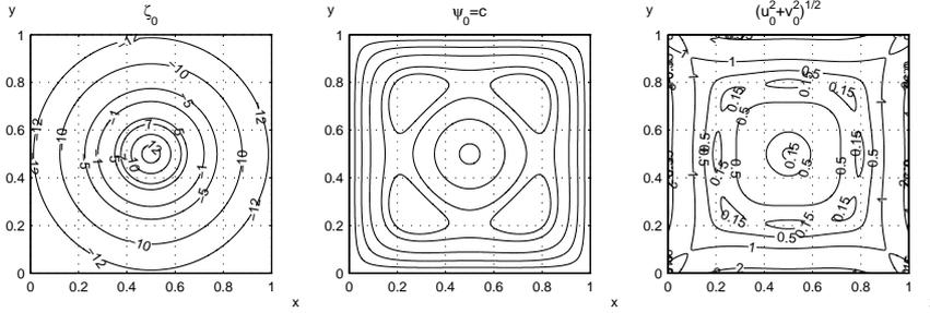
Figure 2. Exponential initial vortex (2.2) at  $t = 0$ . This example is chosen because the vorticity of simple concentric circles induces strong wall velocities while they only produce weak shears near the centre. This is a good case to examine the vorticity production at solid boundaries.
