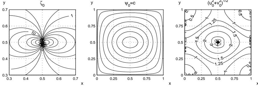
Figure 4. Cat’s-eye initial data (2.4). The core vorticity is stronger and gives rise to a maximum velocity  $|\mathbf{u}_0| \approx 4$  (incompressible). Because of the high core velocity, the wall layers are “thickened” to accommodate the non-slip condition. There is a narrow region next to each wall over which the local velocity is suppressed to zero. Vorticity contours are 0.25, 1, 5, 10, 20, 50, 100 and 250.
