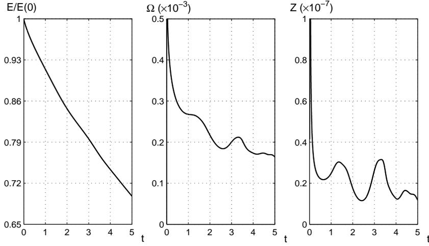
Figure 12. The integrated quantities reflect the developing history of the pair in the preceding figure. The oscillations in the enstrophy or palinstrophy are closely related to the birth and re-birth of the small vortices. As a monitoring parameter, we find that the circulation  $\Gamma \sim O(10^{-15}) \forall t > 0$ . In addition, mesh convergence is examined at  $n = 1024$  and  $n = 1280$ .
