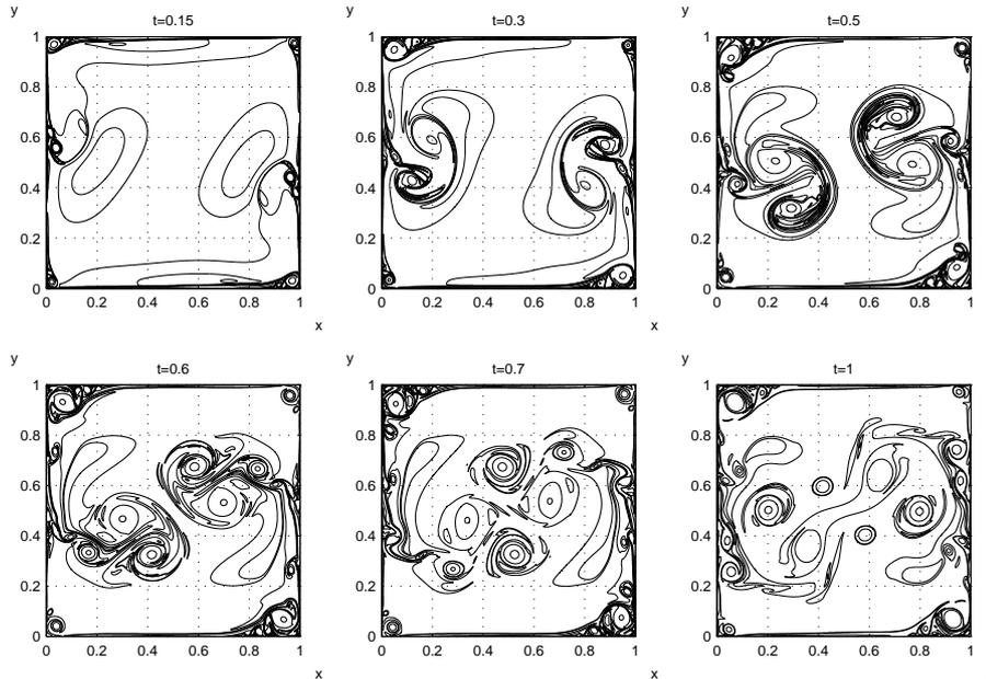
Figure 17. Evolution of data (2.5) over time. Plotted vorticity contours are  $-250, -70, -10, -5, 20, 50$  and  $100$ . The vorticity has strong disparate gradients on the two side walls. Preliminary test runs indicate that high mesh density is crucial in revealing the fine-scale details, both before and after the collision. The simulation captures the broad features of the head-on impact, cf. the flow visualisation on p.24 of Samimy *et al.* (2004).
