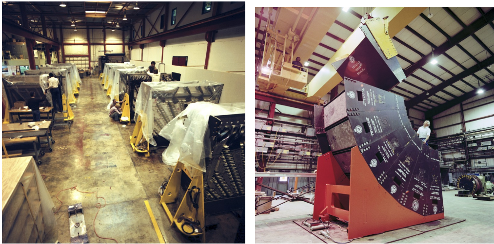
Figure 18: Left: Franco Cervelli and Aldo Menzione working on hadron calorimeter modules. Right: Hans Kautsky supervising the assembly of prototype ‘arch’ of modules being assembled at Argonne. (Note the hard-hat).
