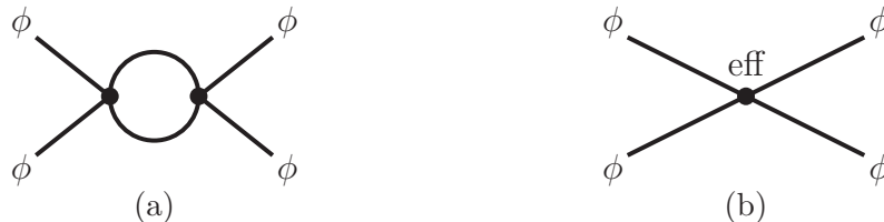
Figure 2: (a) one-loop diagram at high energy in a full theory. (b) its corresponding vertex diagram in its EFT at low energy when locality is restored.
