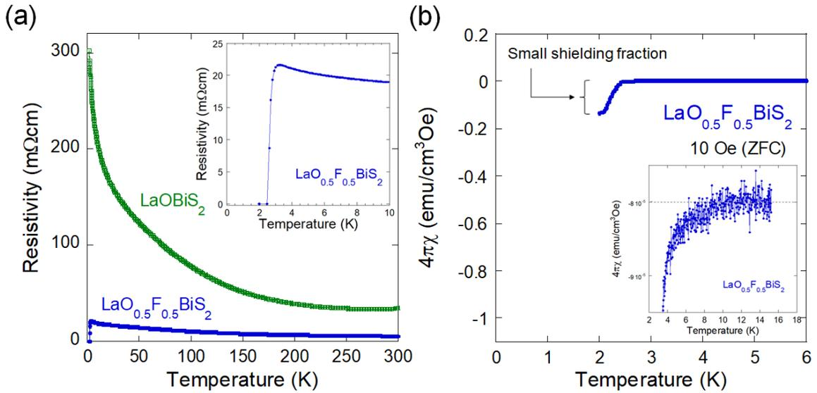
Fig. 4. (Color online) Temperature dependences of (a) electrical resistivity and (b) magnetic susceptibility of  $\text{LaOBiS}_2$  and  $\text{LaO}_{0.5}\text{F}_{0.5}\text{BiS}_2$ . The original data was partly published in Ref. 13.
