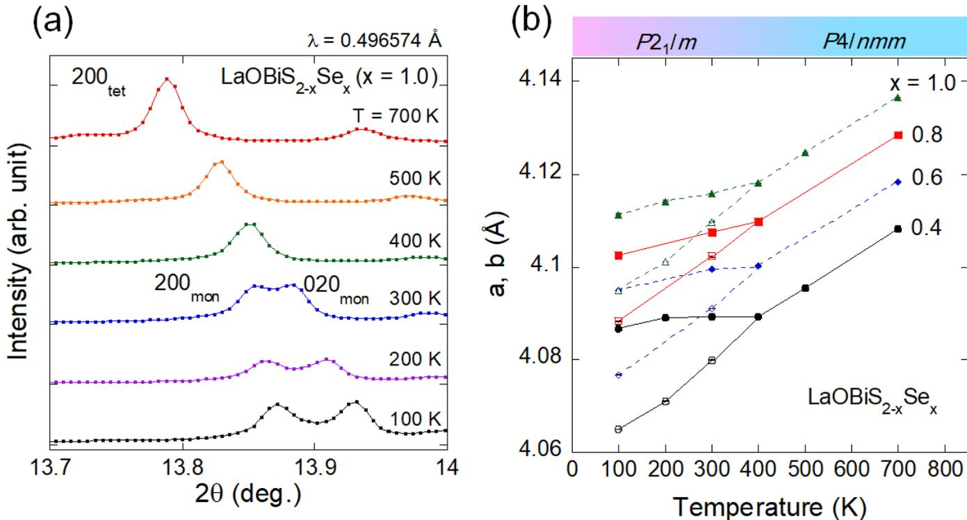
Fig. 7. (Color online) (a) Temperature dependence of synchrotron X-ray profile near the 200 peak of LaOBiS<sub>2-x</sub>Se<sub>x</sub> for  $x = 1.0$ . Tet and mon denote tetragonal and monoclinic, respectively. (b) Temperature dependences of lattice parameters for LaOBiS<sub>2-x</sub>Se<sub>x</sub>.
