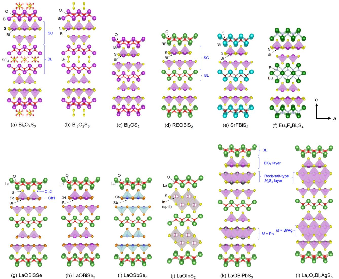
Fig. 1. (Color online) Schematic images of the crystal structure of BiS<sub>2</sub>-based and related materials. The crystal structure images were prepared using VESTA software [220]. SC and BL denote superconducting and blocking layers, respectively.
