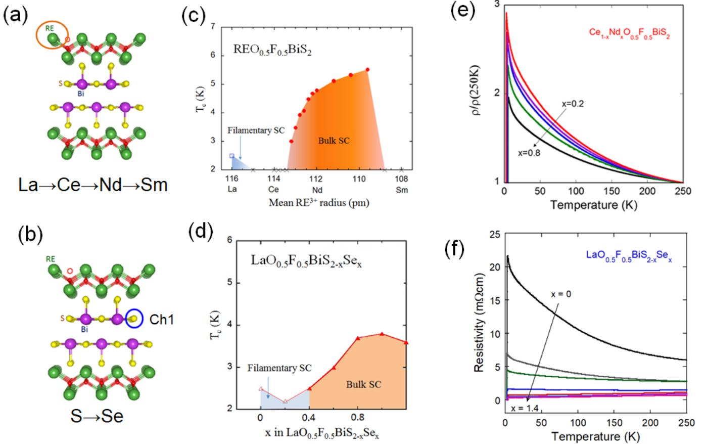
Fig. 9. (Color online) (a) Schematic image of RE site substitution. (b) Schematic image of Se substitution for the in-plane Ch1 site. (c,d) Superconductivity phase diagram for  $\text{REO}_{0.5}\text{F}_{0.5}\text{BiS}_2$  and  $\text{LaO}_{0.5}\text{F}_{0.5}\text{BiS}_{2-x}\text{Se}_x$ . SC denotes superconductivity. (e,f) Temperature dependences of normalized resistivity for  $\text{REO}_{0.5}\text{F}_{0.5}\text{BiS}_2$  and  $\text{LaO}_{0.5}\text{F}_{0.5}\text{BiS}_{2-x}\text{Se}_x$ .
