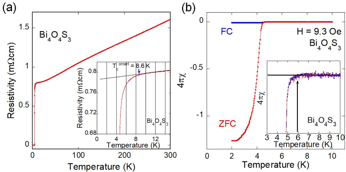
Fig. 2. (Color online) Temperature dependences of (a) electrical resistivity and (b) magnetic susceptibility of Bi<sub>4</sub>O<sub>4</sub>S<sub>3</sub>. The original data was partly published in Ref. 12.
