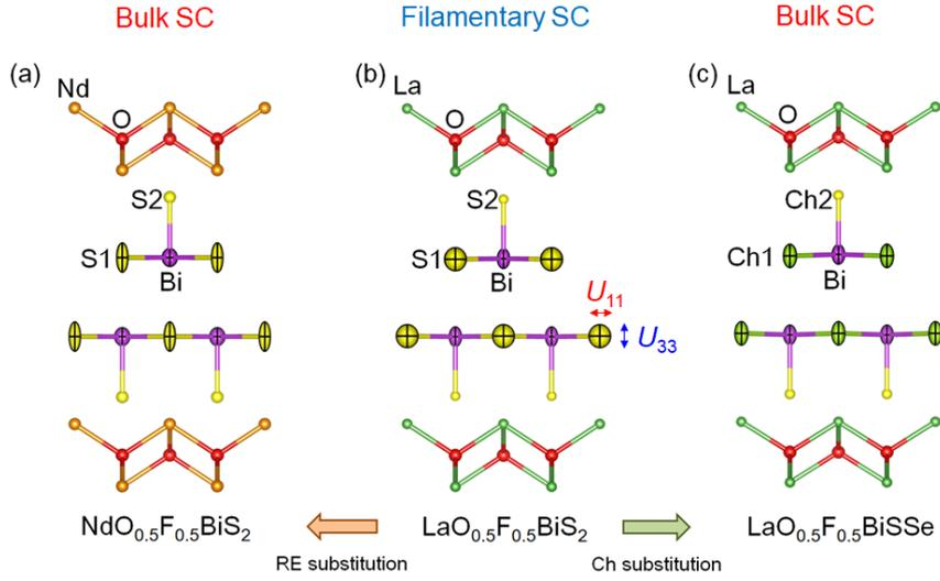
Fig. 13. (Color online) Schematic images of CP effect and anisotropic displacement parameters. The displacement ellipsoids depict the 90% probability. The images were drawn using VESTA.
