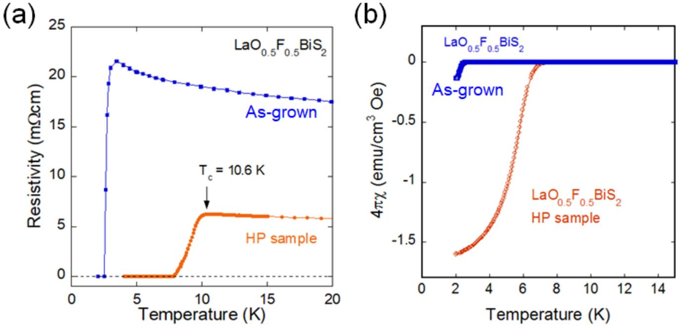
Fig. 5. (Color online) Temperature dependences of (a) electrical resistivity and (b) magnetic susceptibility for as-grown and HP-annealed samples of  $\text{LaO}_{0.5}\text{F}_{0.5}\text{BiS}_2$ . The original data was partly published in Ref. 13.
