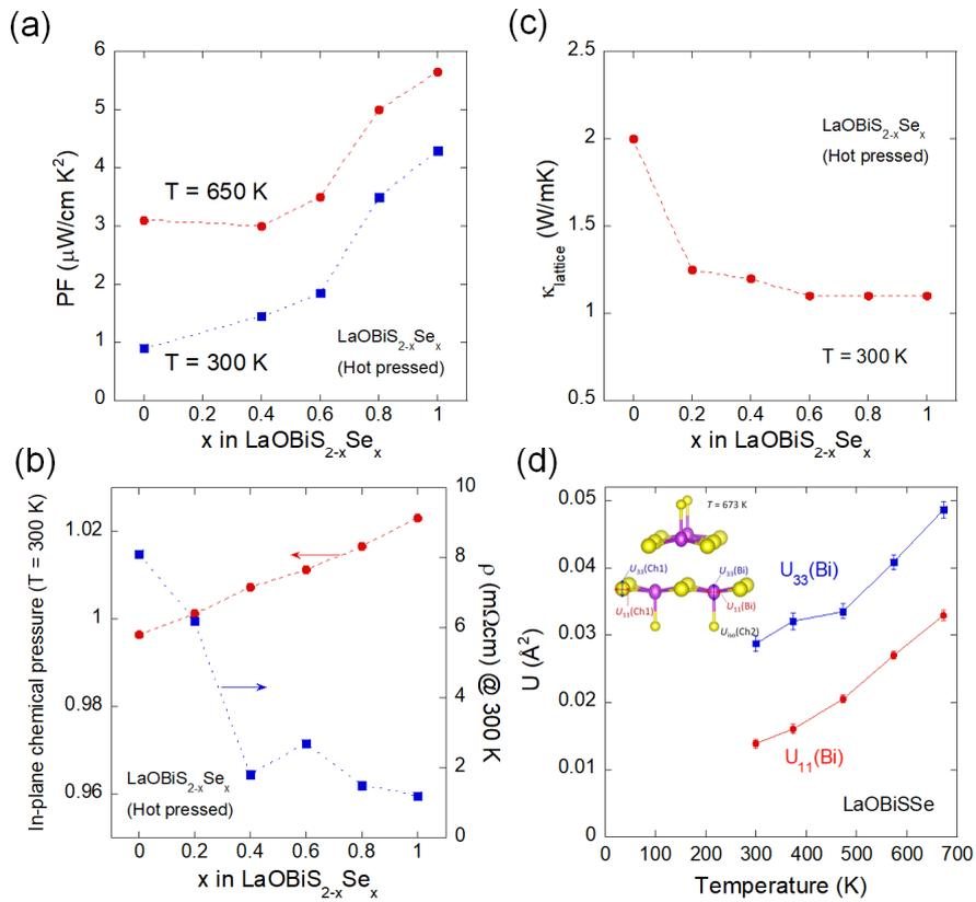
Fig. 14. (Color online) (a–c) Se concentration dependences of  $PF$ , in-plane CP,  $\rho$ , and  $\kappa_{\text{lattice}}$  for  $\text{LaOBiS}_{2-x}\text{Se}_x$ . (d) Temperature dependences of  $U_{11}$  and  $U_{33}$  for Bi. The original data was partly published in Refs. 162, 166, and 207.
