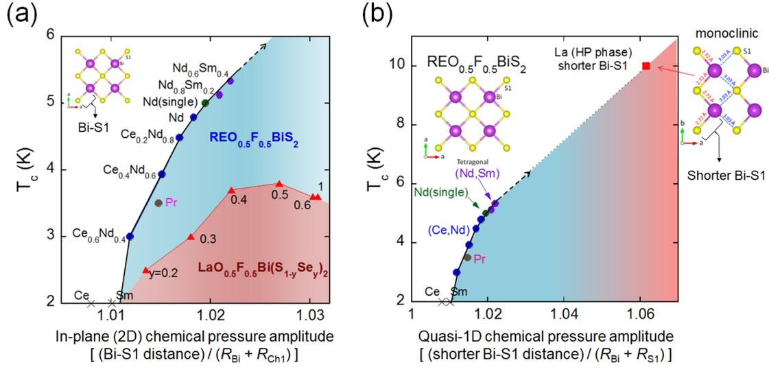
Fig. 11. (Color online) Superconductivity phase diagrams for  $\text{REO}_{0.5}\text{F}_{0.5}\text{BiS}_2$  and  $\text{LaO}_{0.5}\text{F}_{0.5}\text{BiS}_{2-x}\text{Se}_x$  as functions of (a) in-plane (2D) CP amplitude (estimated using the equation described at the bottom) and (b) quasi-one-dimensional CP amplitude. The original data was partly published in Ref. 141. 2D and 1D denote two- and one-dimensional, respectively.
