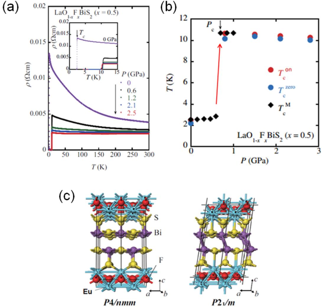
Fig. 6. (Color online) (a) Temperature dependences of electrical resistivity for  $\text{LaO}_{0.5}\text{F}_{0.5}\text{BiS}_2$  under high pressure. (b) Pressure dependence of  $T_c$  for  $\text{LaO}_{0.5}\text{F}_{0.5}\text{BiS}_2$ . (c) Schematic image of structural transition from tetragonal  $P4/nmm$  to monoclinic  $P2_1/m$  by pressure effect. Reproduced from Tomita et al., J. Phys. Soc. Jpn. 83, 063704 (2014). [81]. ©[2014] The Physical Society of Japan.
