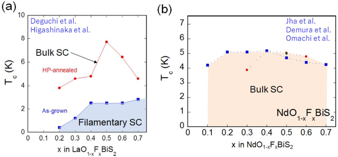
Fig. 8. (Color online) Superconductivity phase diagram for (a)  $\text{LaO}_{1-x}\text{F}_x\text{BiS}_2$  and (b)  $\text{NdO}_{1-x}\text{F}_x\text{BiS}_2$ . The original data were partly published in Refs. 17, 46, 50, 85, and 138. SC denotes superconductivity.
