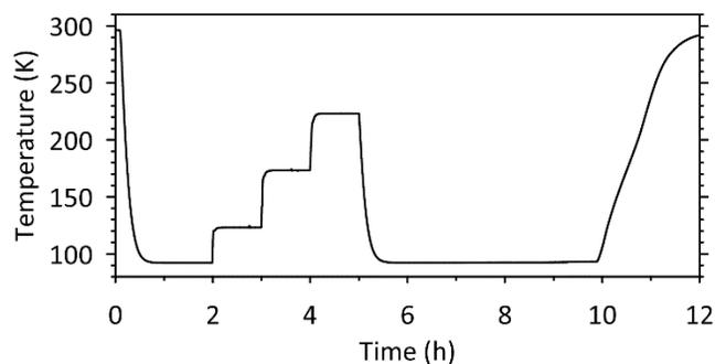
**Figure 5:** Temperature profile of the Gatan 630 sample holder while loaded in the cryo-STXM at  $10^{-8}$  Torr.
