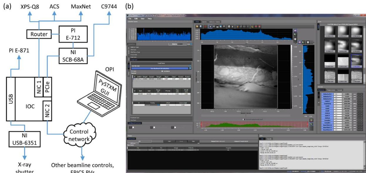
**Figure 4:** (a) Block diagram depicting the control system. (b) Screen capture of the graphical user interface of the control program, pySTXM.
