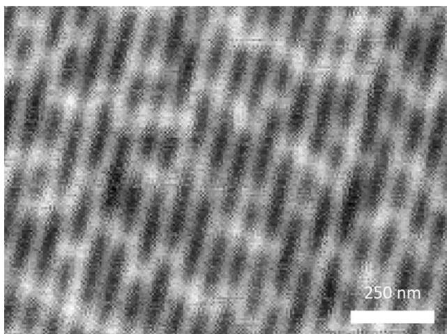
**Figure 8:** X-ray transmission image at 694.0 eV of 35 nm outermost zones of a gold ZP, acquired at 92 K and  $10^{-9}$  Torr.
