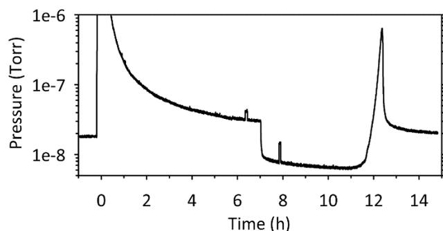
**Figure 6:** Pumpdown curve in goniometer mode, no bake out.
