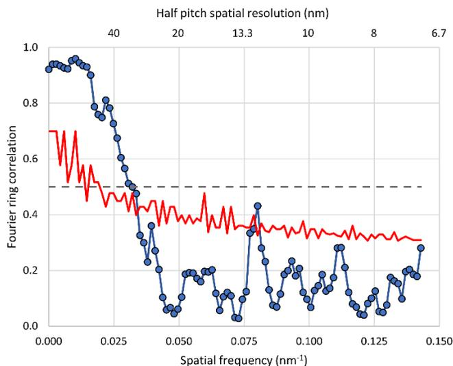
Fourier ring correlation (FRC) analysis of the image presented in Figure 8. The blue data points are the FRC. The dashed grey line represents the 0.5 threshold, and the FRC crosses the 0.5 threshold at a spatial frequency corresponding to a half pitch spatial resolution of 31 nm. The red line is the half-bit threshold, and the FRC crosses the half-bit threshold at a spatial frequency corresponding to a half pitch spatial resolution of 29 nm.
