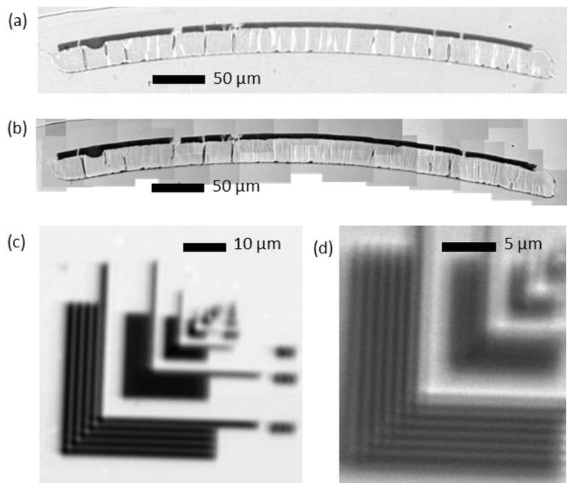
A) Conventional full field optical microscope image (Olympus BX51) of a polymer electrolyte membrane hydrogen fuel cell thin section ( $100\times$  total magnification, transmission using a white light source). The optically transparent membrane region is on the bottom while the relatively opaque and thinner cathode region is on top.
