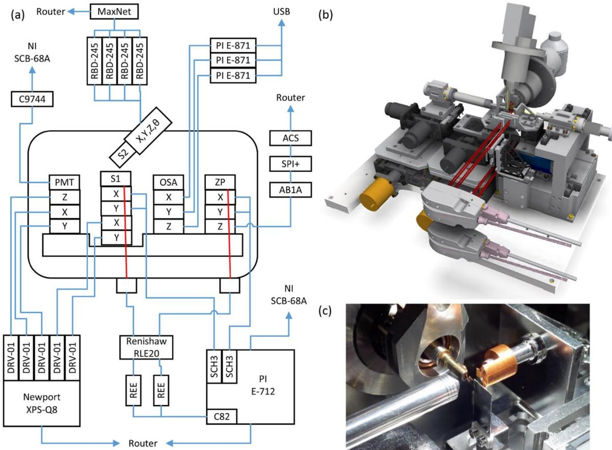
**Figure 3:** (a) Block diagram depicting the stage layout along with drivers and controllers. (b) 3D CAD model of the instrument with the vacuum chamber removed. (c) Photograph inside the vacuum chamber (outboard side view) in goniometer mode. Beam enters from the right in all sub-panels.
