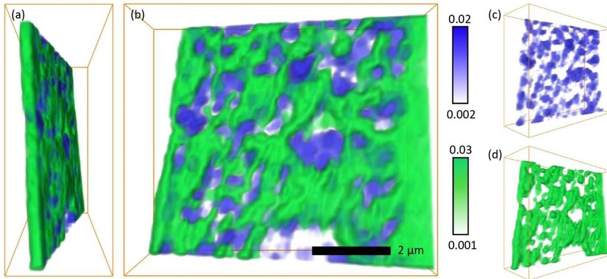
**Figure 11:** 4D volume rendered images of a PEM fuel cell thin section, with PFSA in green and carbon support in blue, (a) Z-Y view, and (b) X-Y view. Individual spectrotomographs of (c) carbon support and (d) PFSA. Otsu threshold [71] values were 0.001 in the range of 0-0.03 for PFSA, 0.002 in the range 0-0.02 for carbon support.
