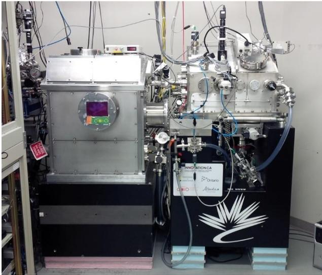
**Figure 1:** Photograph of the inboard side of the soft X-ray STXMs at the CLS SM beamline, ambient-STXM (left, upstream) and cryo-STXM (right, downstream).
