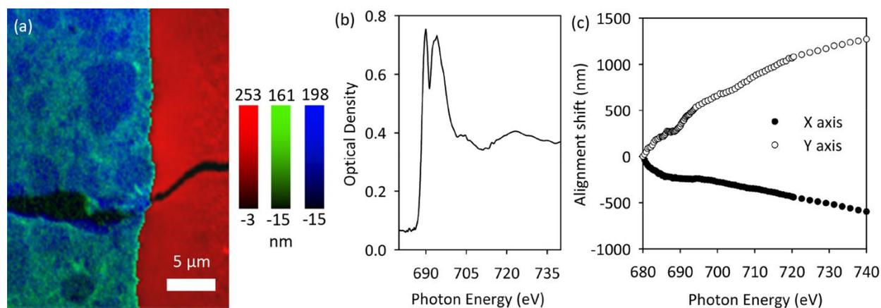
**Figure 9.** Results derived from a F 1s stack of a PEM fuel cell sample. (a) Color coded composite of thickness maps in nanometers of compounds in the sample: PFSA in the membrane in red, PFSA in the cathode in green, and carbon support in the cathode in blue. (b) F 1s XANES spectrum derived from the membrane region. (c) The post-exposure alignment file for the stack of 92 images.
