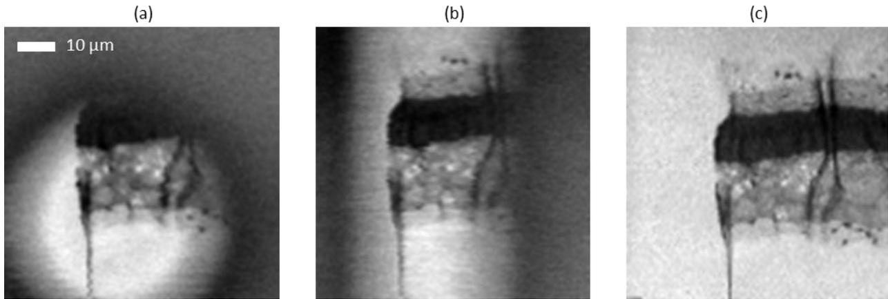
A) ZP fly scanning with a stationary OSA. The diameter of the bright area is  $70\ \mu\text{m}$ , which is equal to the diameter of the OSA. This scan mode is generally used when the desired field of view is less than the difference between the diameter of the ZP central stop and the diameter of the OSA, typically less than  $20\ \mu\text{m} \times 20\ \mu\text{m}$ .
