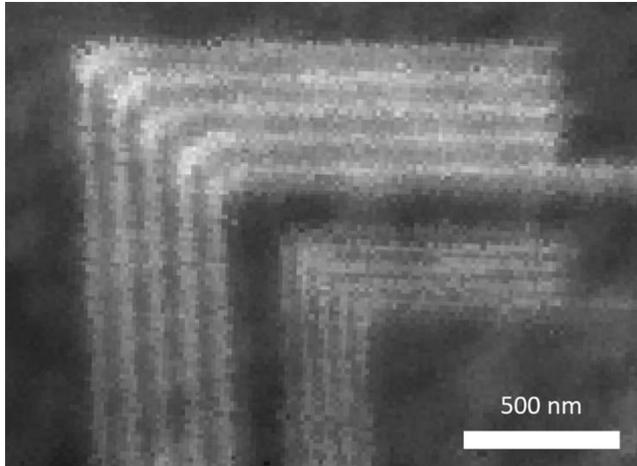
**Figure 7:** X-ray transmission image at 395.0 eV of a resolution test pattern with 50 nm and 30 nm half pitch elbows, acquired at 296 K and  $10^{-2}$  Torr.
