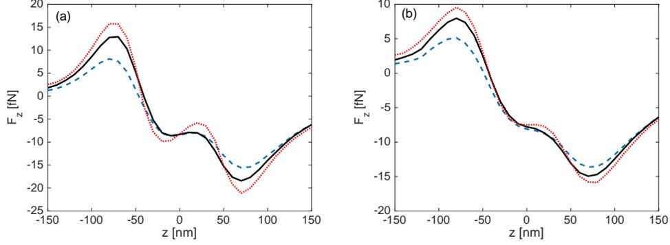
FIG. 7. Optical force exerted upon a 50nm-radius polystyrene nanoparticle along  $z$ -direction at (a)  $x=100\text{nm}$  (b)  $x=90\text{nm}$  from the center of the hole. (Red-dotted) Maxwell stress tensor, (solid black) dipole approximation including the backaction effect, (blue-dashed) conventional dipole approximation without considering the backaction effect.
