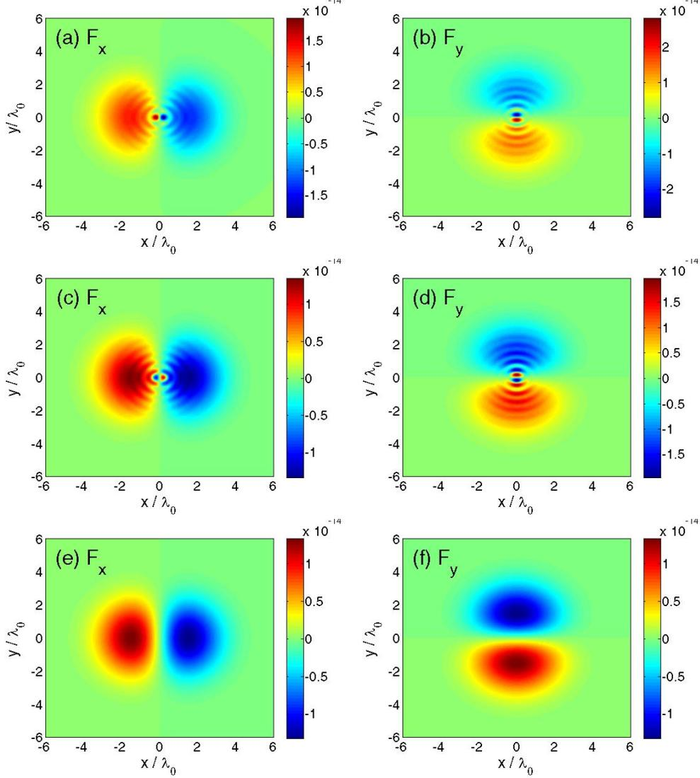
FIG. 2. Optical force exerted upon a 110 nm nanosphere with refractive index 2.5 at the  $z = 0$  plane. (a),(b) For  $R_0 = (2n - 1)\frac{\lambda_0}{4}$ . (c),(d) For  $R_0 = (2n + 1)\frac{\lambda_0}{4}$ . (e),(f) In the absence of the spherical mirror. These results are obtained for  $I_0 = 2[\frac{mW}{\mu m^2}]$  and  $w_0 = 3\lambda_0$
