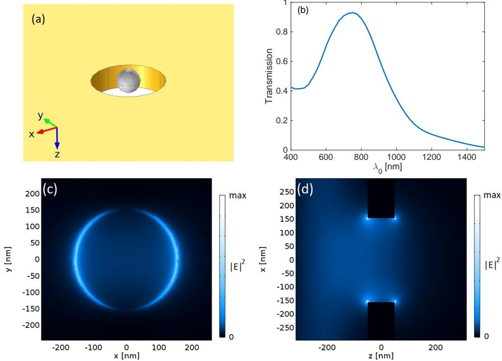
FIG. 5. (a) Schematic of the CNH structure. (b) Transmission spectrum of CNH structure in the absence of the nanosphere. (c), (d) Intensity profiles of the electromagnetic fields in the absence of the nanosphere.
