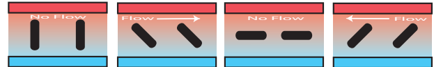
FIG. 14: Sketch of the four consecutive configurations of a generator of alternating flow, in which states of no-flow, and flow with positive and negative directions can periodically alternate.
