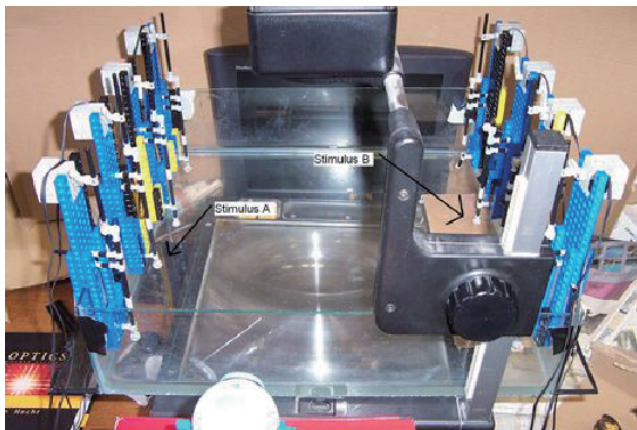
Figure 2: A fluidic RC where the reservoir is the water in a bucket (Fernando and Sojakka, 2003). Figure reproduced with permission from Springer Nature.
