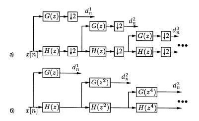
**Fig 4. Two types of the filter bank for a discrete wavelet transform.** (top) Mall's algorithm. (bottom) Algorithm á trous.
