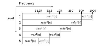
Fig 5. Detailed coefficients of the discrete wavelet transform. Detailed coefficients characterize the different frequency ranges for the scales k = 1, 2, 3, 4, 5 at a signal sampling frequency of 1000 Hz. *wac* means "wavelet approximation coefficients", *wdc* means "wavelet detailed coefficients".
