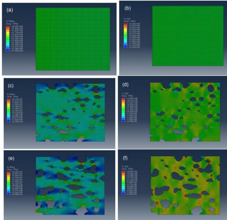
Figure 4: Vin-Mises stress of media with (a) no porosity (c) 10% porosity (e) 20% porosity and stress perpendicular to the direction of subjected load with (b) no porosity (d) 10% porosity (f) 20% porosity
