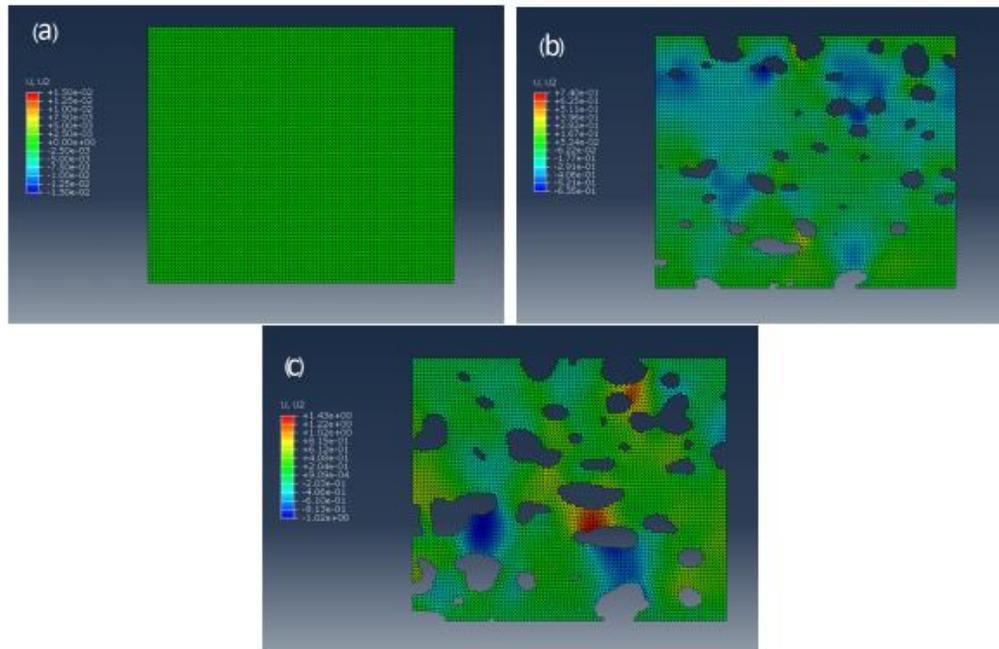
Figure 3: deformation perpendicular to the direction of subjected load with (a) no porosity (b) 10% porosity (c) 20% porosity.
