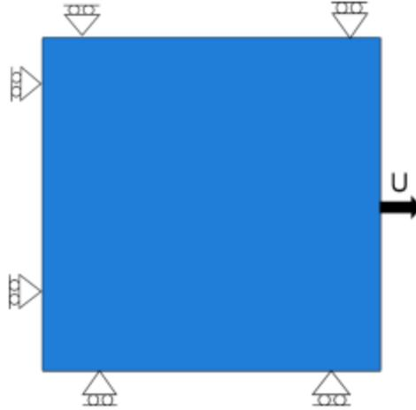
Figure 2: Schematic boundary condition of finite element model.
