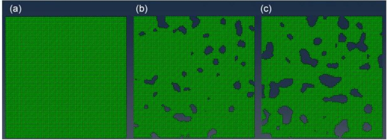
Figure 1: (a) nonporous media, (b) porous media with 10% porosity, and (c) porous media with 20% porosity.
