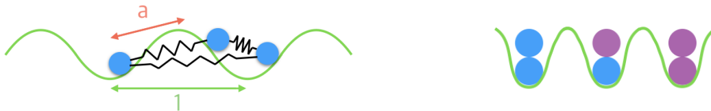
Figure 2: Left : The Frenkel-Kontorova model. Particles are linked by springs with positive equilibrium length a , and subject to an external potential of period L (set here to 1). The competition between springs and external potential leads to symmetry breaking, i.e. the preferred distance between particle 1 and 2 is different from that between particle 2 and 3. Right : Ground state of the total spring energy of an ensemble of 3-particle molecules when the external potential is replaced by rigid confinement to three consecutive minima and we impose the constraint that each minimum must be occupied by the same number of particles. This is precisely the multi-marginal optimal transport problem from Example 1.1.
