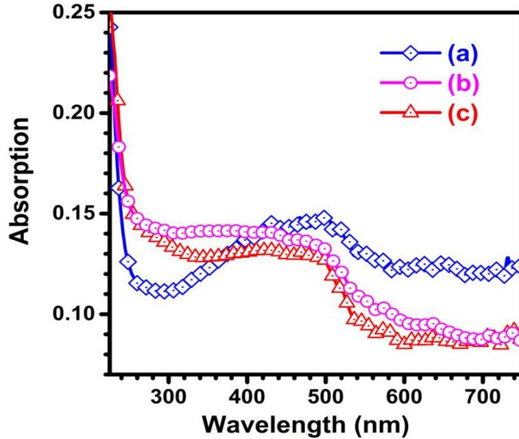
Fig. 4. Comparison of absorption peak arising from defects of three different ZnS NPs a) 3 nm, b) 3.5 nm, c) 4.5 nm. Inset shows variation of absorption at 500 nm with concentration.
