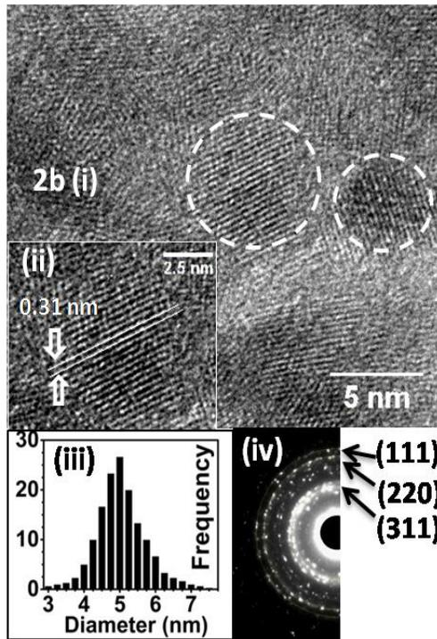
Fig. 2b. HRTEM studies elucidating typical, (i) Quantum sized ZnS synthesized from 0.5 wt% ZnCl<sub>2</sub>, (ii) the *d* spacing of the (111) plane of cubic ZnS phase, (iii) particle size distribution with a maximum around 5 nm and (iv) SAED pattern confirming cubic phase of ZnS.
