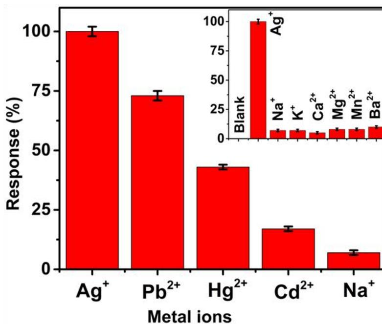
Fig. 10. Response of metal ions to 3 nm ZnS NPs with reference to 100% response for Ag<sup>+</sup>. The inset displays the selectivity of Ag<sup>+</sup> with respect to alkali and alkaline metals which most expected to present in aquatic medium.
