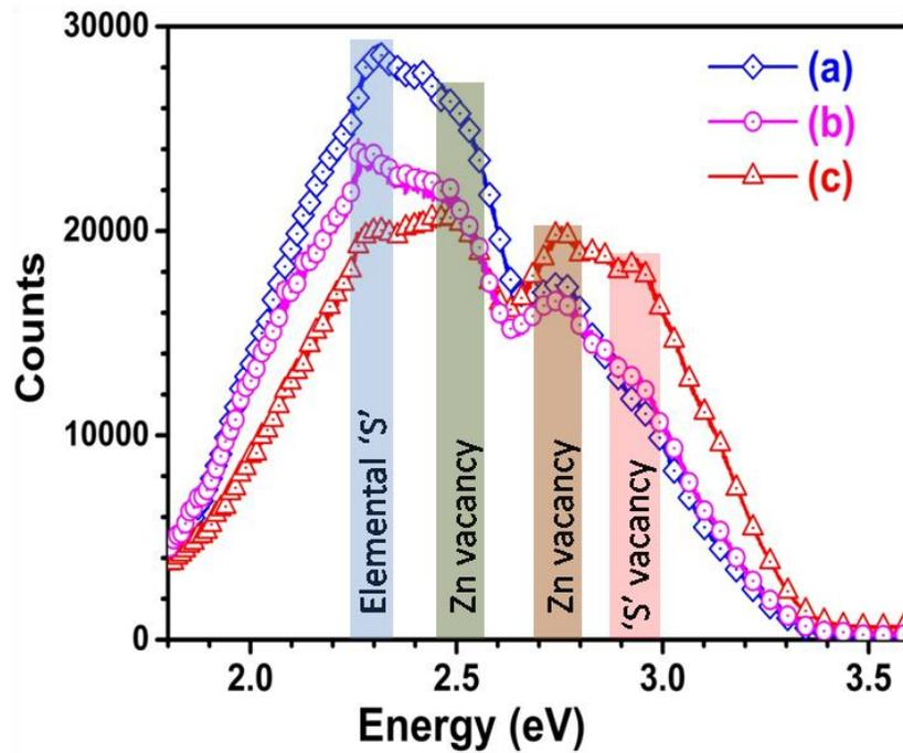
Fig. 5. PL spectra showing presence of defects in ZnS NPs a) 3 nm, b) 3.5 nm, c) 4.5 nm.
