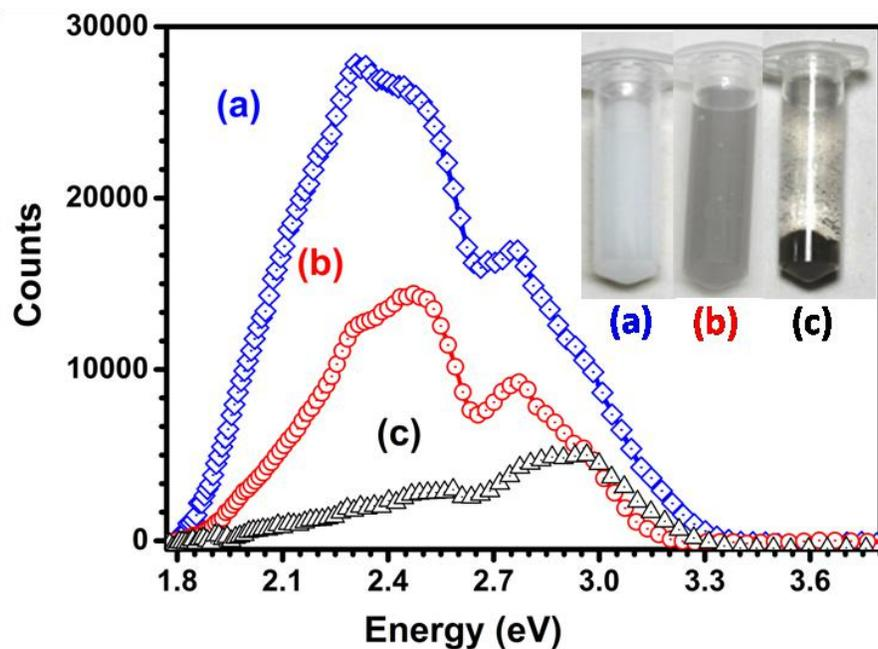
Fig. 8. Typical PL spectra recorded before and after addition of AgNO<sub>3</sub> to 3 nm ZnS NPs, a) ZnS NPs, b) with 1 μM AgNO<sub>3</sub>, c) with 1 mM AgNO<sub>3</sub>. Each tube in the inset displays a) ZnS NPs, b) ZnS NPs with 1 μM AgNO<sub>3</sub>, c) ZnS NPs with 1 mM AgNO<sub>3</sub>.
