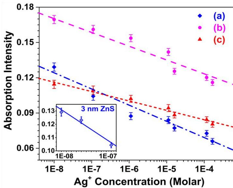
Fig. 7. Optimized response at 500 nm for three different particle sizes. Response curve for a) 3 nm, b) 3.5 nm, c) 4.5 nm ZnS. The inset displays linear variation of response for very low concentrations of  $\text{Ag}^+$ .
