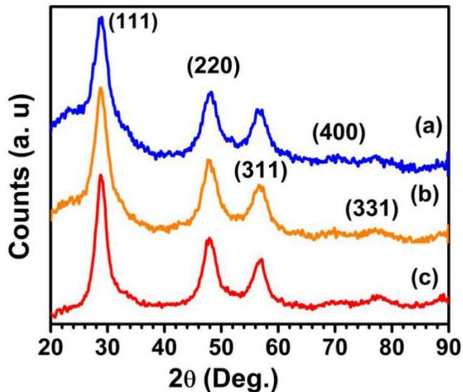
Fig. 1. XRD of various ZnS NPs prepared with concentrations of ZnCl<sub>2</sub> a) 0.1 wt% b) 0.25 wt% and c) 0.5 wt%.
