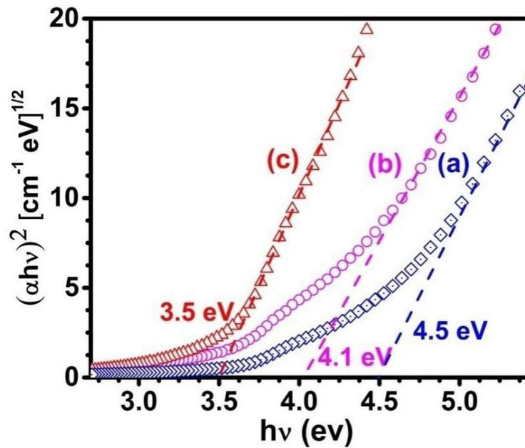
Fig. 3. Tauc's plot for different sizes of ZnS NPs, a) size 3 nm, b) size 3.5 nm, c) size 4.5 nm. Smaller size particle exhibits higher band gap due to quantum confinement effect.
