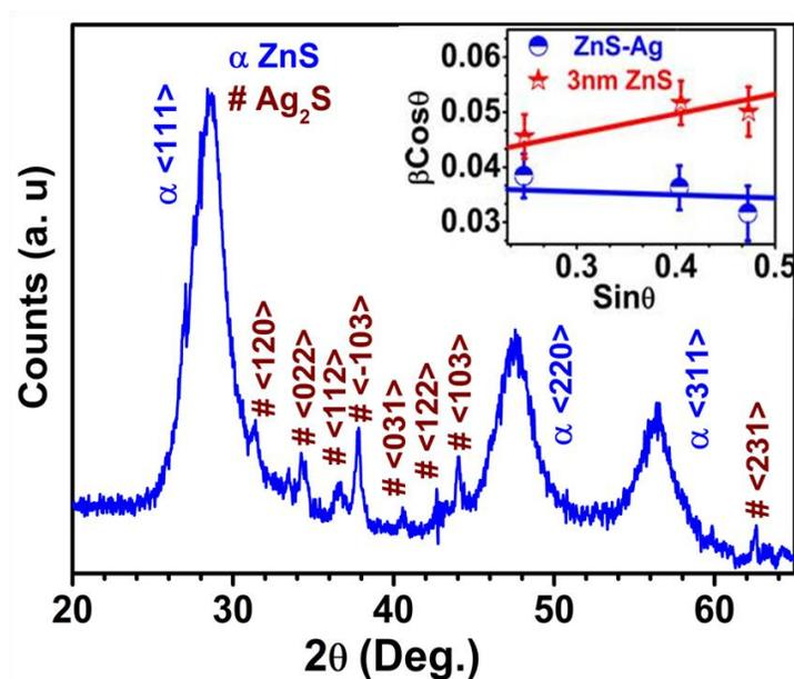
Fig. 9. XRD of ZnS NPs after reaction with AgNO<sub>3</sub> solution. The inset is W-H plot for the smallest ZnS NPs (3 nm) and the ZnS NPs after addition of AgNO<sub>3</sub>.
