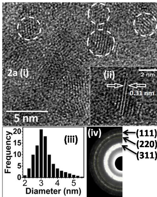
Fig. 2a. HRTEM studies elucidating (i) quantum sized ZnS synthesized from 0.1 wt% ZnCl<sub>2</sub>, (ii) the *d* spacing of the (111) plane of cubic ZnS phase, (iii) particle size distribution with a maximum around 3 nm and (iv) SAED pattern confirming cubic phase of ZnS.
