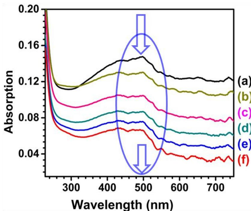
Fig. 6. UV-Vis absorption spectra for a) pure ZnS in water and with the addition of different concentrations of  $\text{AgNO}_3$  b) 10 nM, c) 0.1  $\mu\text{M}$ , d) 1  $\mu\text{M}$ , e) 50  $\mu\text{M}$ , f) 0.5 mM.
