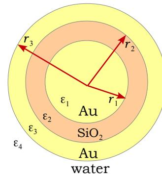
FIG. 1. (Color online) Schematic illustration of gold nanomatryoshkas.
