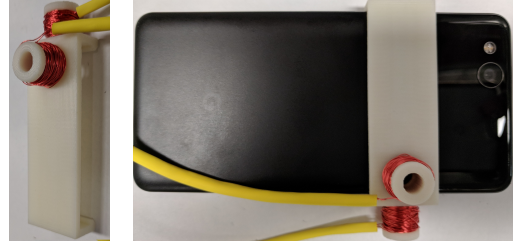
(b) The two-coil system attached to a Google Pixel 2
