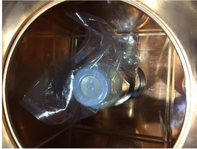
Fig. 2 Picture of the HPGe measurement for 500 g of \text{Gd}_2(\text{SO}_4)_3 \cdot 8\text{H}_2\text{O} .
