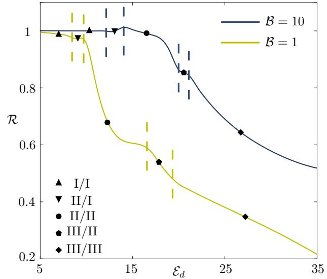
FIG. 3. The liquid absorption ratio,  $\mathcal{R}$ , of permeable sheets compared to impermeable ones of the same  $\mathcal{E}_d$  for  $\mathcal{B} = 1$  and  $\mathcal{B} = 10$ . Dashed lines separate the different combinations of equilibrium regimes for permeable and impermeable cases and symbols denote the regimes (e.g., II/I indicates that permeable sheets reach regime II while impermeable sheets are at regime I).
