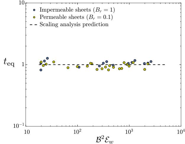
FIG. 4. Time to reach the 99% of the equilibrium height versus  $\mathcal{B}^2 \mathcal{E}_w$ . Symbols represent the numerical results for the equilibrium time scale of impermeable and permeable sheets. The dashed line indicates  $t_{\text{eq}} = 1$ .
