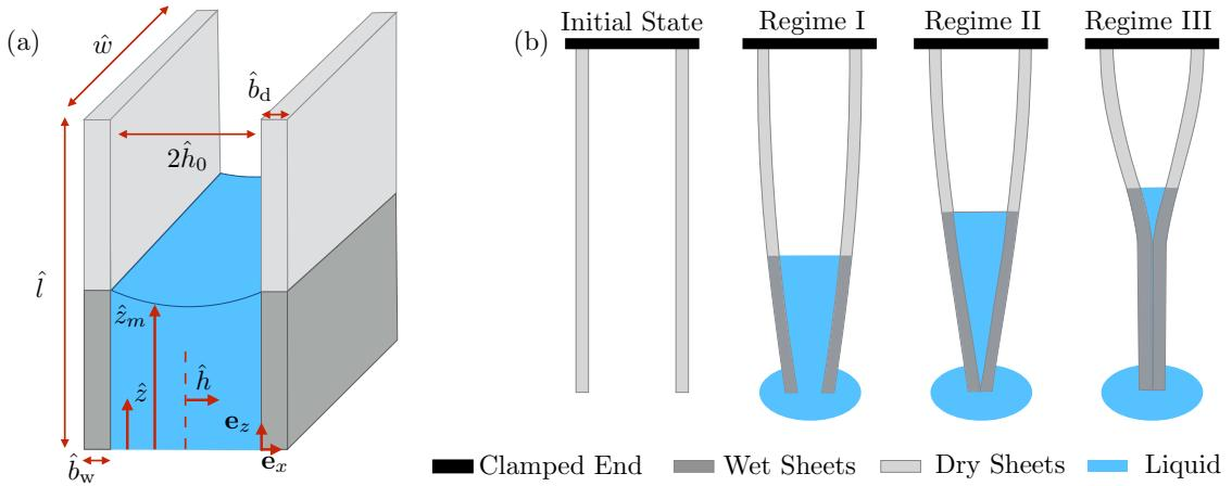
FIG. 1. The schematic of the system: (a) Two poroelastic sheets clamped at the upper end are immersed into a liquid bath from the lower end. (b) Three scenarios of the equilibrium. In regime I, sheets only slightly bend. In regime II, sheets lower end are in contact and in regime III, sheets coalesce over a finite length.
