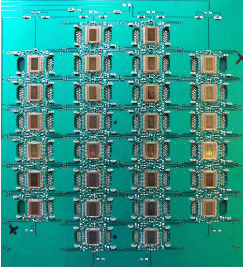
**Figure 6.** Photograph of the digital side of an 896-channel (28-chip) readout assembly. This larger system demonstrated scalability of the pixelated readout design, and was used to fully instrument and operate a 10-cm-diameter LArTPC.
