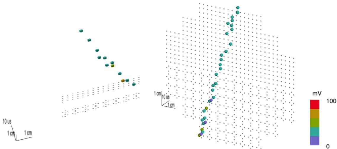
**Figure 8.** *Left:* 3D image of a cosmic ray muon which passed at a steep angle relative to the face of a 128-channel readout system. *Right:* A similar image of a cosmic ray muon passing nearly coplanar to a fully-instrumented 832-channel readout system. Both figures display the raw data generated by the readout system; no filtering or signal enhancement has been applied.
