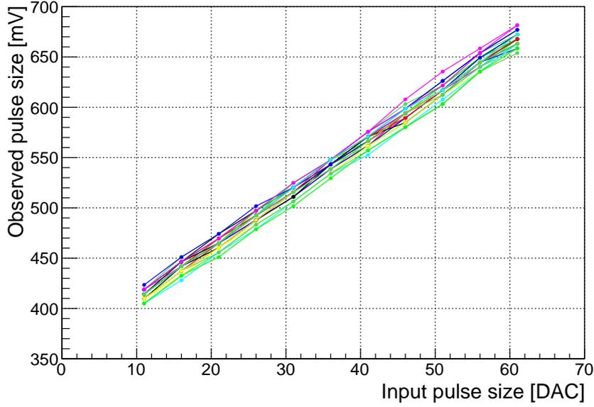
**Figure 4.** Plot of the self-triggered ADC value versus internal pulser DAC value for the 32 channels of one LArPix ASIC. The slope of each line provides a preliminary assessment of the CSA gain, consistent with the design specification of  $4 \mu\text{V}$  per electron. The digital ADC value has been converted to voltage based on an initial calibration of the ADC scale.
