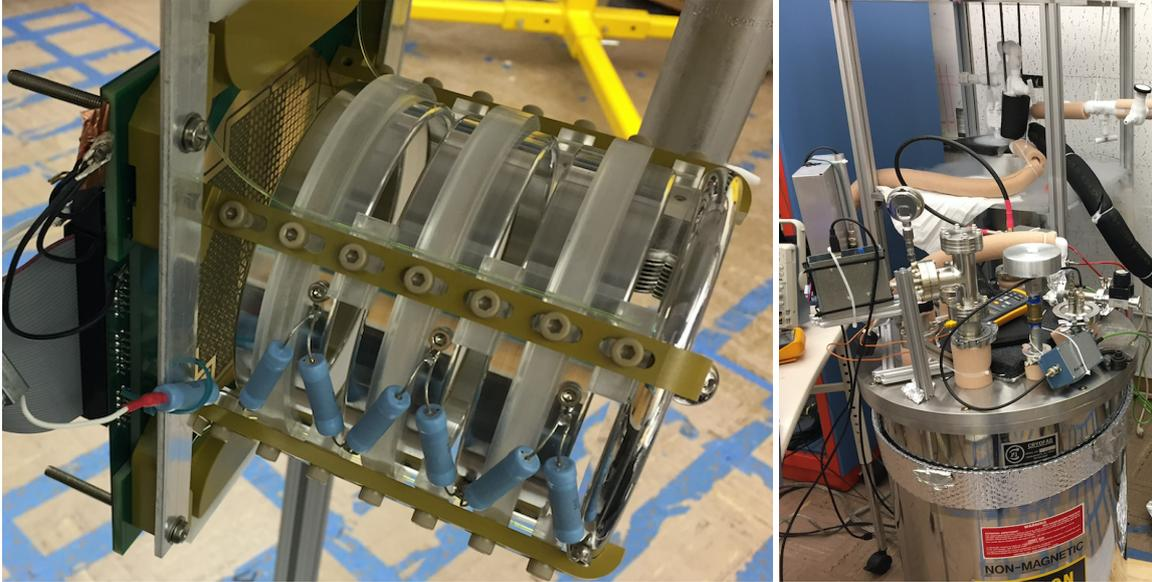
**Figure 7.** *Left:* Photograph of the 10-cm-drift TPC with a 3D readout system installed. *Right:* Photograph of the high-purity liquid argon system during operation. The TPC is installed in the cryostat (foreground). A single-pass of research-grade liquid argon through the LAr purifier (background) is sufficient to achieve electron lifetimes in excess of  $100 \mu\text{s}$ .
