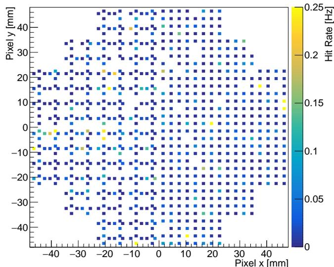
**Figure 9.** Channel self-trigger rates for an 832-channel pixelated readout system with 3 mm spacing. The majority of channels have low rates ( $\sim 0.02$  Hz) that are dominated by the cosmic ray signals of interest. A few channels have low thresholds and high rates ( $> 0.05$  Hz) that are primarily noise. A few-percent of channels were disabled due to high noise rates, and are visible as gaps in the pixelated array.
