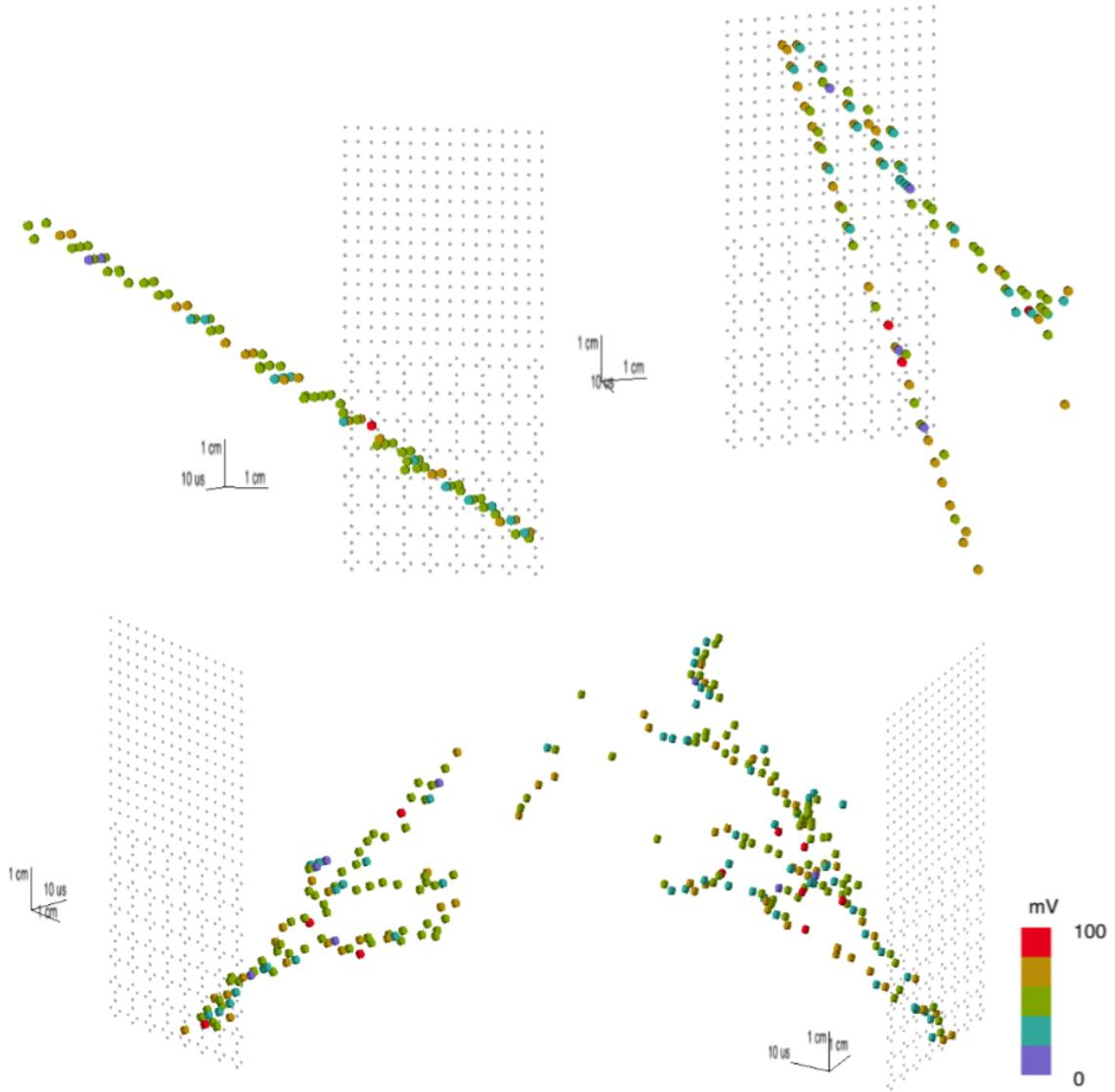
**Figure 10.** Four example 3D images of cosmic ray interactions detected using a 4.8 cm by 9.6 cm readout system in a 60-cm-drift LArTPC. The upper figures show relatively simple straight muon tracks, while the lower figures show small electromagnetic showers. This is raw data collected from the system; no filtering or enhancement has been applied.
