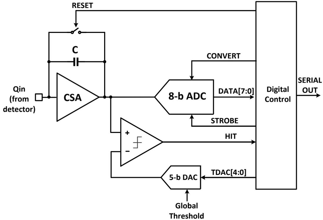
**Figure 1.** Block diagram of the LArPix application-specific integrated circuit (ASIC).
