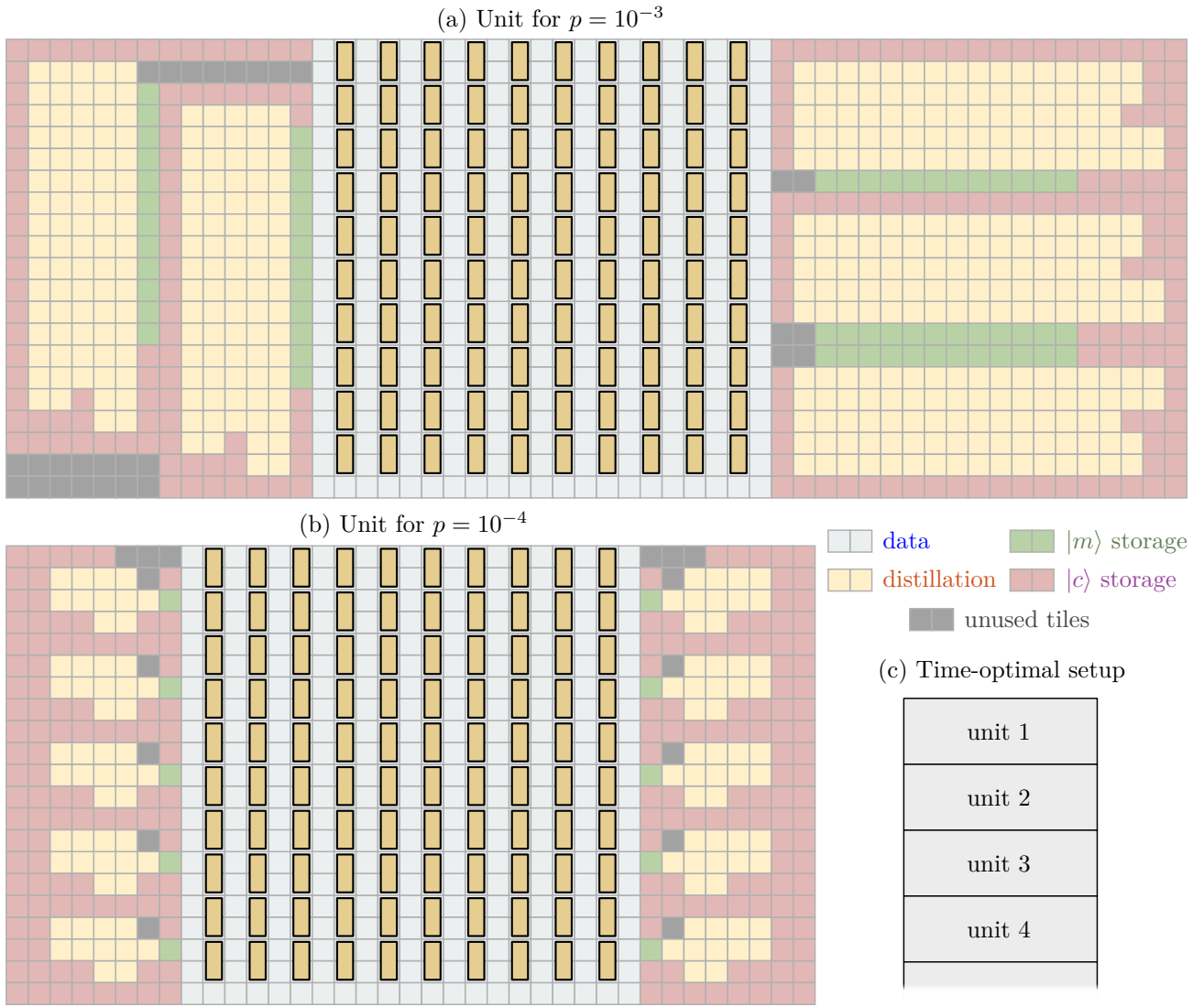
Figure 29: Units consist of fast data blocks, modified distillation blocks and storage tiles. (a) The unit for p = 10^{-3} consists of 54 \times 21 = 1134 tiles. (b) For p = 10^{-4} , the number of tiles is 37 \times 21 = 777 . (c) A time-optimal setup consists of a row of multiple units, which means that the space to the bottom and top of the fast data blocks needs to remain free.
