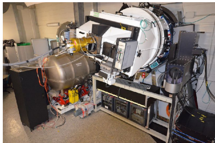
Figure 8. The GIARPS configuration at the Nasmyth-B focus of TNG. Left: The electronics and the dewar containing GIANO-B: the latter is mounted on a dedicated platform attached to the telescope fork. Bottom center: The new GIANO-B pre-slit (black box) and the corresponding electronics. Right: The front-end and calibration units of HARPS-N. GIANO-B and HARPS-N receive the NIR and VIS light beams separated by a dichroic, hosted by LRS (Low Resolution Spectrograph, top center). Credit: TNG-Fundación Galileo Galilei.
