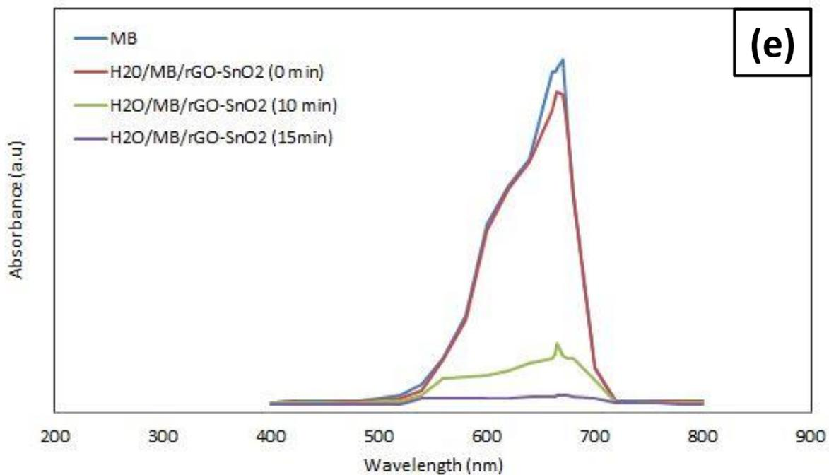
Fig. 7: Time-dependent absorption spectra of MB solution during UV light irradiation in the presence (a) GO, (b) SnO<sub>2</sub>, (c) GO-SnO<sub>2</sub>, (d) rGO and (e) rGO-SnO<sub>2</sub>
