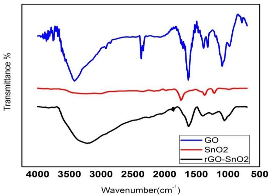
Fig. 4: FTIR curves of GO, SnO<sub>2</sub> and rGO-SnO<sub>2</sub>
