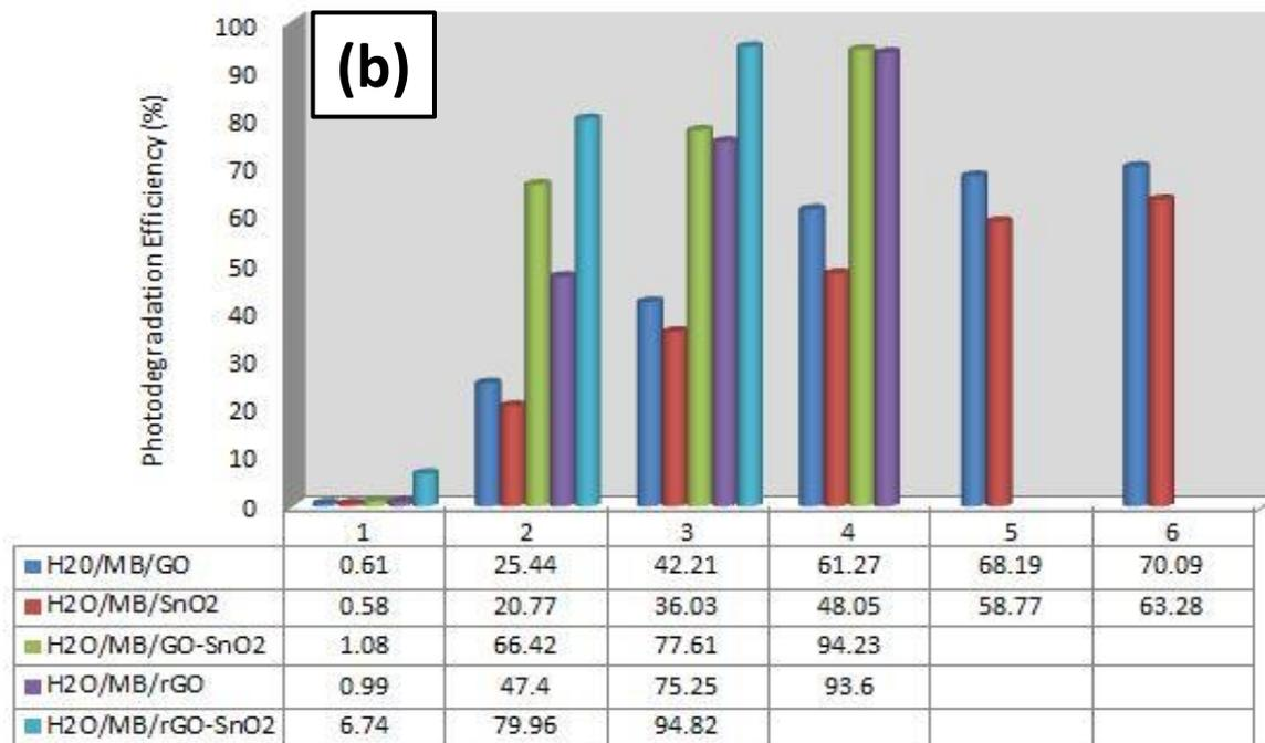
Fig. 9: Photodegradation Efficiency (%) under (a) Natural Sunlight and (b) UV light
