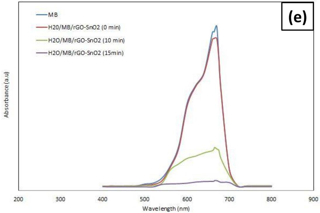
Fig. 5: Time-dependent absorption spectra of MB solution during natural sunlight irradiation in the presence (a) GO, (b) SnO<sub>2</sub>, (c) GO-SnO<sub>2</sub>, (d) rGO and (e) rGO-SnO<sub>2</sub>
