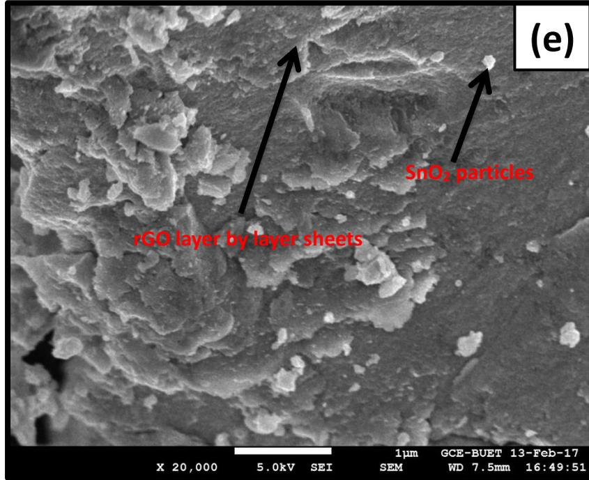
Fig. 2: SEM of (a) GO, (b) SnO<sub>2</sub>, (c,d) GO-SnO<sub>2</sub> and (e) rGO-SnO<sub>2</sub>
