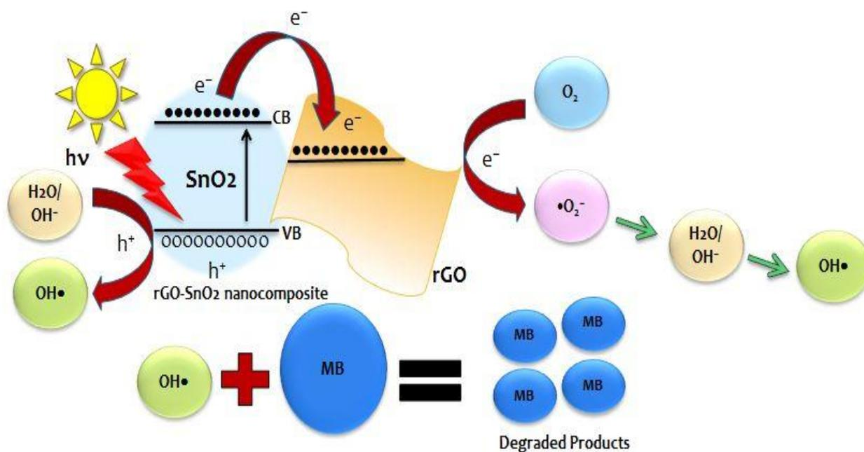
Fig. (A): Photodegradation of MB using rGO-SnO<sub>2</sub> nanocomposite under sunlight irradiation
