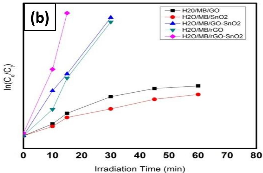
Fig. 8: (a) Absorbance versus Irradiation time curves for GO, SnO<sub>2</sub>, GO-SnO<sub>2</sub>, rGO and rGO-SnO<sub>2</sub> and (b)  $\ln(C_0/C_t)$  versus UV light Irradiation time curves illustrating MB photo degradation by GO, SnO<sub>2</sub>, GO-SnO<sub>2</sub>, rGO and rGO-SnO<sub>2</sub>
