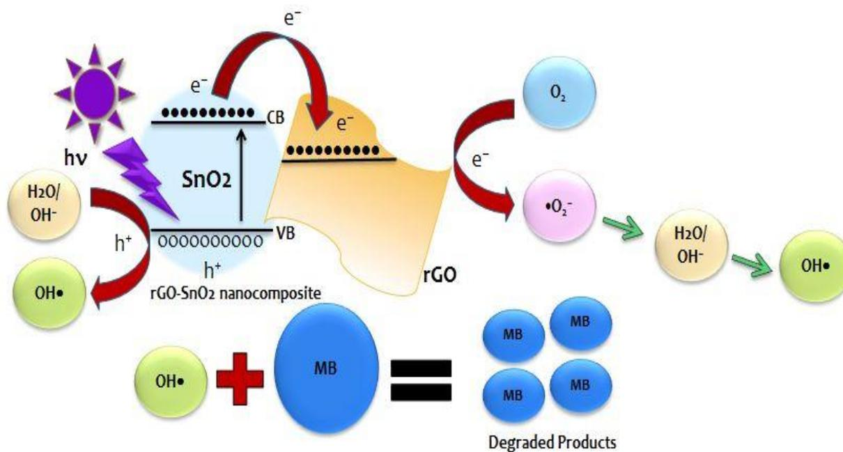
Fig. (B): Photodegradation of MB using rGO-SnO<sub>2</sub> nanocomposite under UV light irradiation
