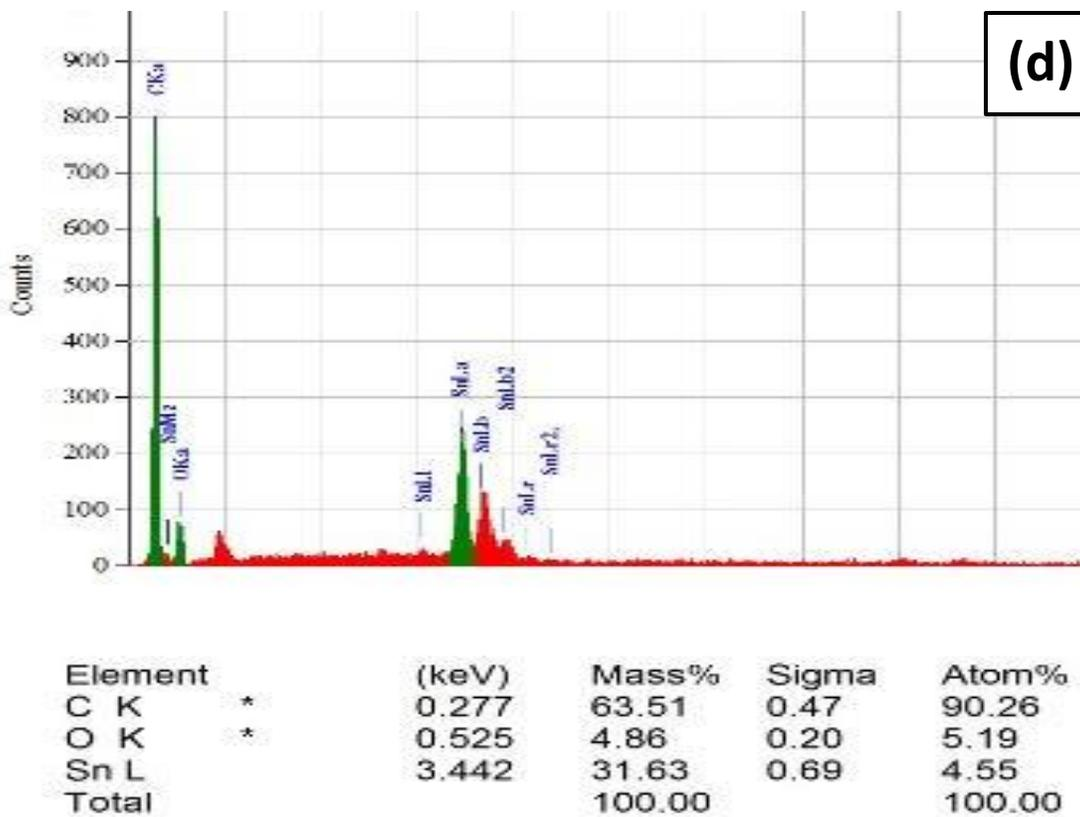
Fig. 3: EDX spectra of (a) GO, (b) SnO<sub>2</sub>, (c) GO-SnO<sub>2</sub> and (d) rGO-SnO<sub>2</sub>
