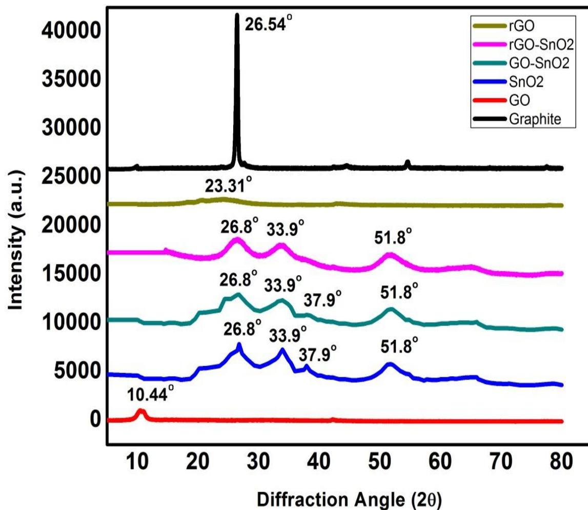
Fig. 1: XRD of Graphite, GO, SnO<sub>2</sub>, GO-SnO<sub>2</sub> and rGO-SnO<sub>2</sub>
