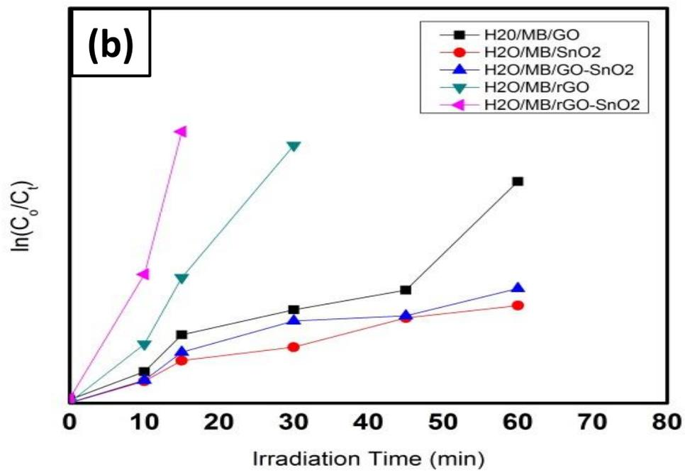
Fig. 6: (a) Absorbance versus Irradiation time curves for GO, SnO<sub>2</sub>, GO-SnO<sub>2</sub>, rGO and rGO-SnO<sub>2</sub> and (b)  $\ln(C_0/C_t)$  versus Irradiation time curves illustrating MB photodegradation by GO, SnO<sub>2</sub>, GO-SnO<sub>2</sub>, rGO and rGO-SnO<sub>2</sub>
