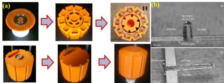
Fig 12. (a) Different stages of hybrid AM of a 3-phase DC motor [169], (b) ink-jet printed actuators with vertical and horizontal morphologies [177].
