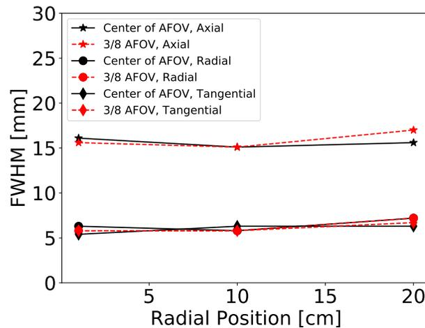
**Figure 12.** Spatial resolution in three directions - the radial, tangential and axial. The geometry was fixed to the single layer chamber with the diameter of 85 cm and strips with length of 50 cm and thickness 7 mm. Hit-time and hit-position resolutions were used as anticipated for the SiPM readout.
