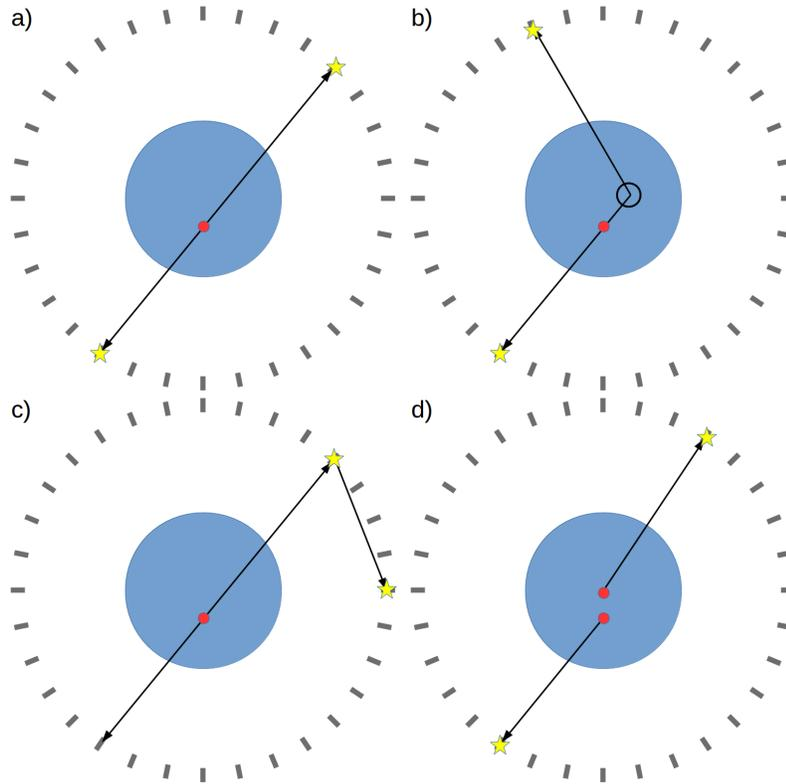
**Figure 4.** Pictorial definitions of different types of coincidences: a) true coincidence, b) phantom-scattered coincidence, c) detector-scattered coincidence and d) accidental coincidence. Blue large circle denotes the phantom, red dots denote the annihilation points, black circle denotes the scattering place in the phantom and yellow stars indicate interactions of gamma photons in the detector.
