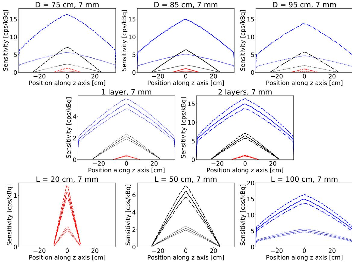
**Figure 11.** Sensitivity profiles grouped by the diameter of the detecting chamber (1st row), number of layers (2nd row) and lengths of the scintillators (3rd row). Legend: D = 75 cm (dashed - -), D = 85 cm (solid -), D = 95 cm (dashed-dotted -.-), 1 layer (thin lines), 2 layers (thick lines), L = 20 cm (red), L = 50 cm (black), L = 100 cm (blue).
