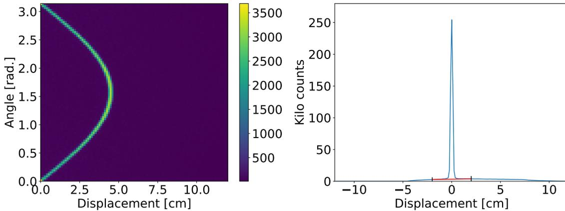
**Figure 9.** Results of the scatter fraction simulation for single-layer geometry with diameter of 85 cm and strips with length of 50 cm. (left) The sinogram for a whole scanner (all slices summed). (right) One dimensional profile calculated as an aligned to zero using maximum value and summed projections of sinogram presented in left panel. The cut level visualized as a red line is determined using values of the profile at  $\pm 2$  cm from zero.
