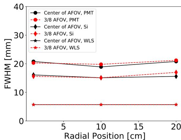
**Figure 13.** Axial resolution for different types of optical photon detectors attached to scintillator strips and two axial positions as a function of radial position of the source. Presented results were obtained for the single-layer geometry with the diameter of 85 cm and strips with length of 50 cm and thickness 7 mm. Note, that the results for WLS at the centre (black stars) and at 3/8 AFOV (red stars) overlap.
