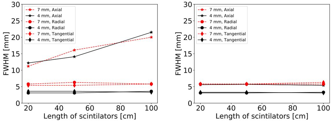
**Figure 14.** Spatial resolution for 3 lengths and 2 thicknesses of scintillator strips assuming readout from silicon photomultipliers (left) and silicon photomultipliers with the WLS strips (right).
