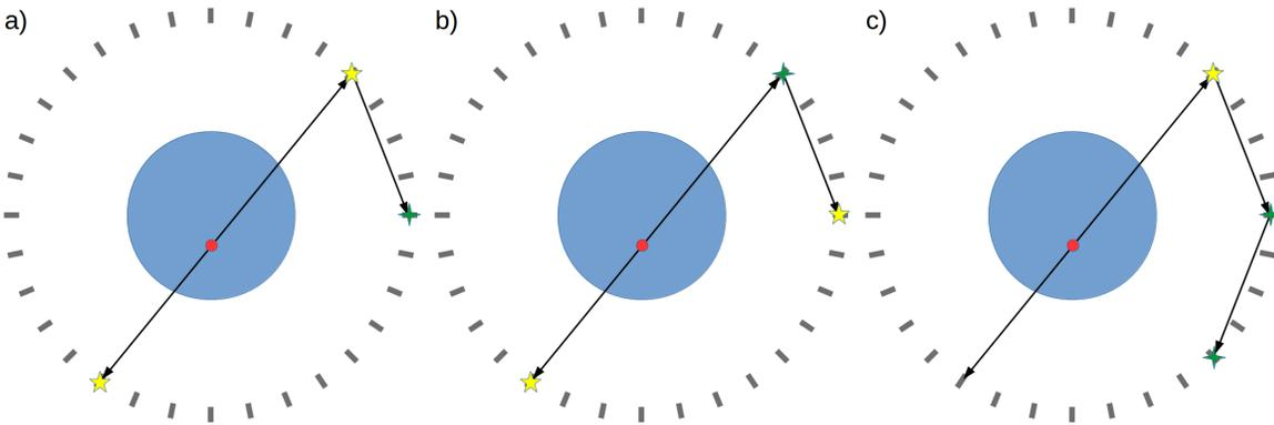
**Figure 5.** Exemplary events with three depositions of energy above the noise threshold: a) true coincidence, b) and c) detector-scattered coincidences. Yellow 5-arm stars visualize depositions of energy bigger than the fixed energy threshold (200 keV) and the green 4-arm stars visualize depositions of energy lower than 200 keV but bigger than the noise energy threshold equal to 10 keV.
