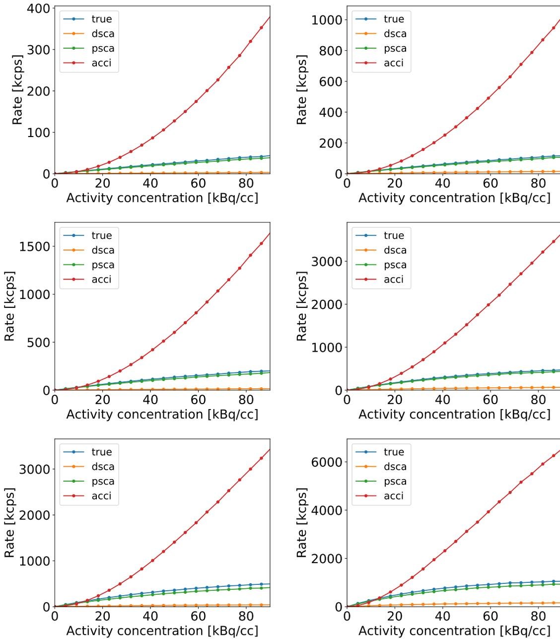
**Figure 16.** Count rates of different types of coincidences for 6 geometries of the J-PET scanner with diameter  $D$  of 85 cm (dsca - detector-scattered, psca - phantom-scattered, acci - accidental coincidences). Left and right panel show results obtained for 1- and 2-layer detectors, respectively. In the first row of the figure, there are rates for 20 cm scintillators, in second row for 50 cm scintillators and in the third row for 100 cm scintillator strips.
