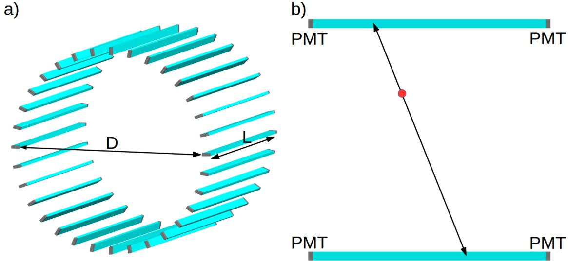
**Figure 1.** a) The exemplary geometry of the J-PET scanner; scintillators are cyan and photomultipliers (PMT) are gray. **D** stands for the diameter of the scanner and **L** the length. For better visualization only 32 strips are shown but in our studies the full angle coverage (without gaps) is used. b) Pair of scintillating strips and two annihilation photons defining the line of response (details in the text). Red point denotes the annihilation point.
