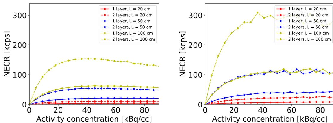
**Figure 17.** Noise equivalent count rate as a function of activity concentration for six geometries of the J-PET scanner. (left) NECR calculated using the true MC rates. (right) NECR calculated using the method based on the sinograms analysis.
