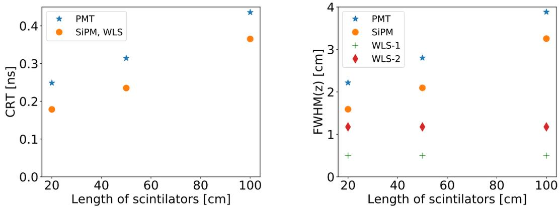
**Figure 3.** The values of CRT (left) and axial resolution (right), used for the simulations, as a function of the length of the scintillator, shown for different readouts [13, 32]. More details are in the text.
