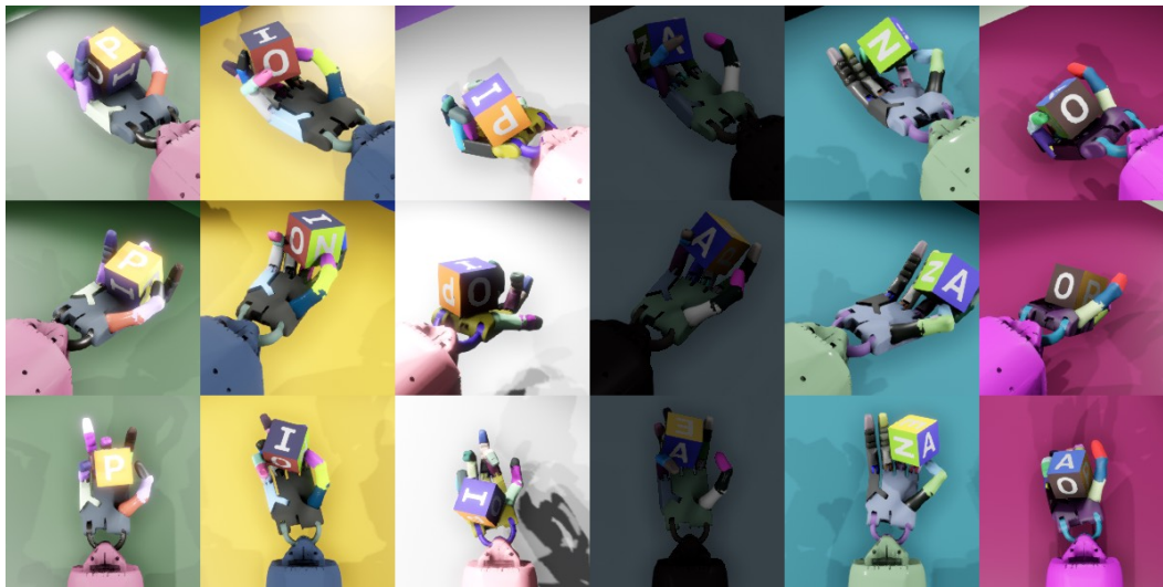
Figure 4: Simulations with different randomized visual appearances. Rows correspond to the renderings from the same camera, and columns correspond to renderings from 3 separate cameras which are simultaneously fed into the neural network.
