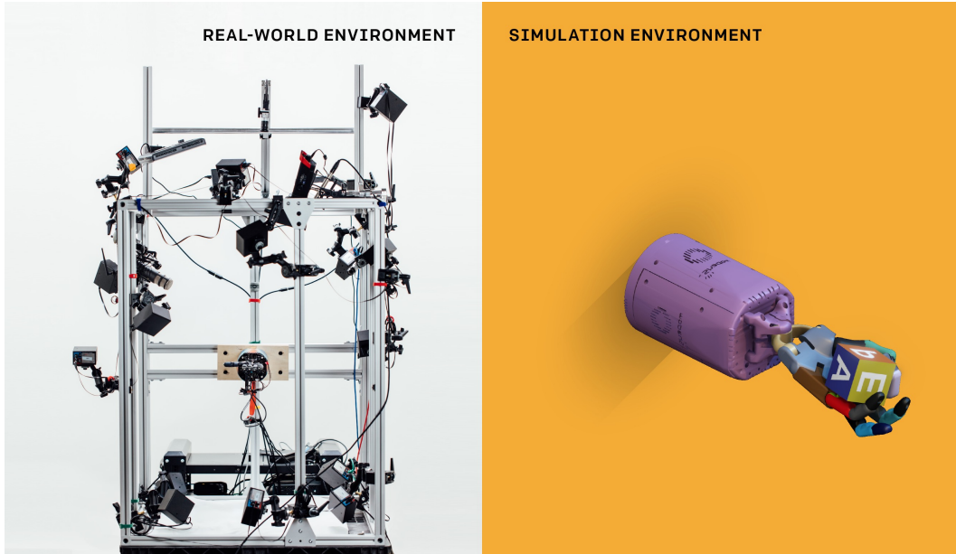
Figure 3: (left) The "cage" which houses the robot hand, 16 PhaseSpace tracking cameras, and 3 Basler RGB cameras. (right) A rendering of the simulated environment.
