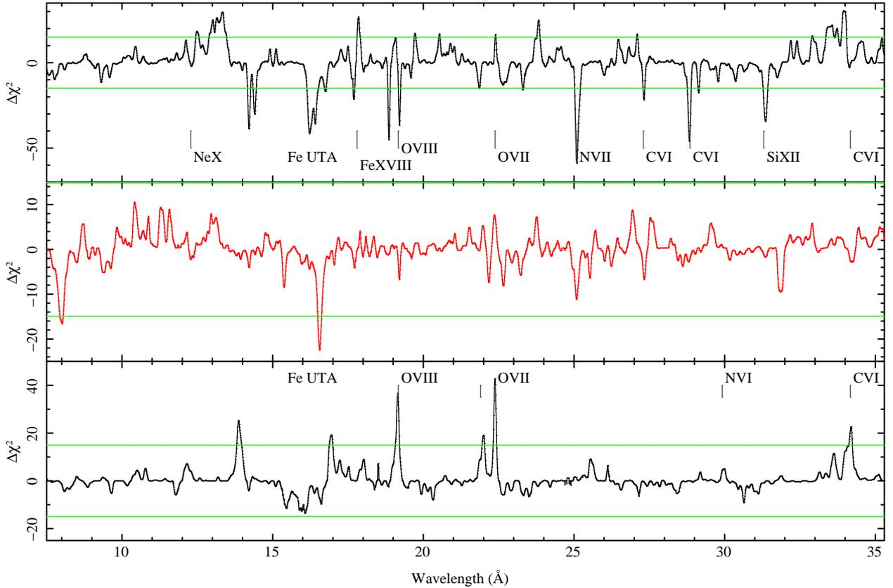
**Figure 6.** Results of line scans to the new data (middle) as well as the highest (top) and lowest (bottom) flux archival observations. The green lines show the 95 % confidence interval for a blind search.
