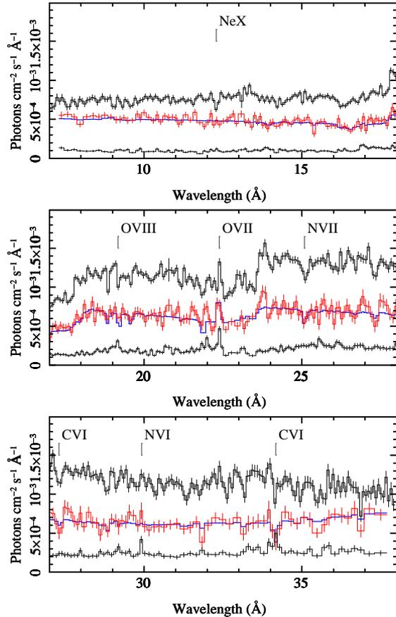
**Figure 5.** RGS data from the new observation (red) and the highest and lowest archival flux states (black) unfolded to a constant model. Emission lines are clearly visible in the low state, while absorption features are present in the high state. The blue line shows a fit with absorption and emission components applied to a phenomenological continuum. Wavelengths are given in the observed frame and the range of each panel overlaps the next by 1 Å.
