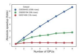
Fig. 1. Speedups obtained using multiple GPUs (GeForce GTX 1080 Ti) for the datasets from Table 1.
