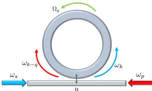
FIG. 3: The ring nanoscale waveguide that is coupled to an external nanofiber with coupling parameter  $u$  that allows tunneling of photons in and out of the waveguide. Inside the waveguide three fields are represented, the photons  $\omega_k$ ,  $\omega_{k-q}$  and the phonon  $\Omega_q$ . Two external fields also appear on the two sides of the external nanofiber, the pump field,  $\omega_p$ , and the signal field,  $\omega_s$ .
