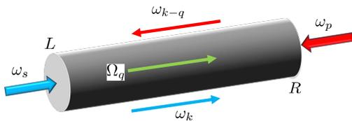
FIG. 2: The linear nanoscale waveguide in which the two sides are considered as two effective mirrors  $L$  and  $R$ , and which allow coupling among external radiation field and internal waveguide field. Inside the waveguide three fields are represented, the photons  $\omega_k$ ,  $\omega_{k-q}$  and the phonon  $\Omega_q$ . Two external fields also appear, the pump field,  $\omega_p$ , on the right, and the signal field,  $\omega_s$ , on the left.
