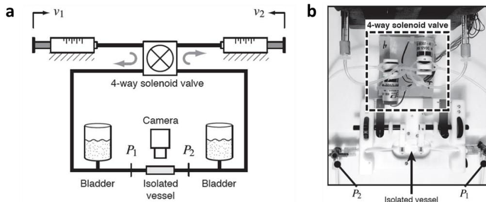
Fig. 6: The vessel perfusion system is shown highlighting the major components. a) The basic control scheme of the perfusion device is shown in the cartoon<sup>54</sup>. The solenoid valves ensure unidirectional flow through the chamber, from the inlet to the outlet. b) The top view shows the tubing connections from the device to the vessel chamber.
