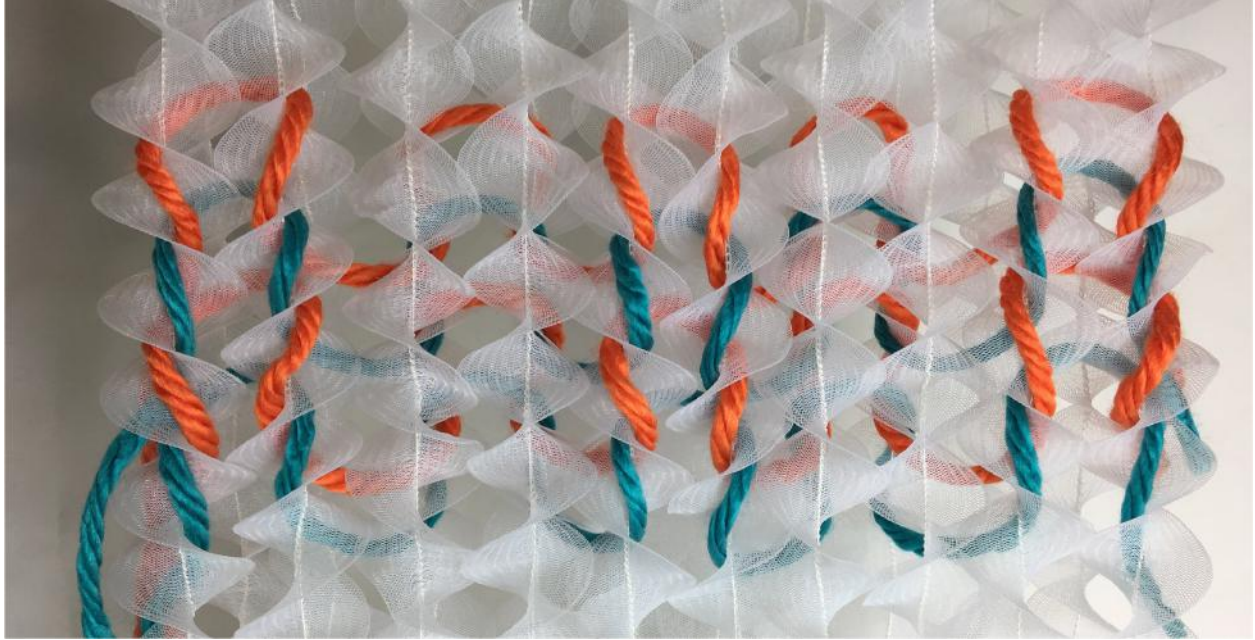
Figure 6. Rib knit structure on the double layer helicoid lattice.
