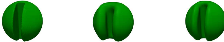
Fig. 3 The 3D Zalesak's disk: the three panels represent the exact initial solution, and those after one full rotation with 33 and 66 grid points per diameter.
