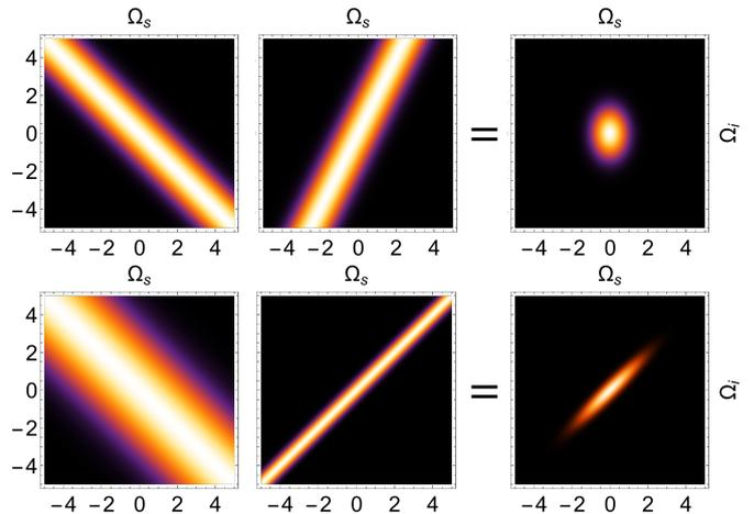
Figure 1. Example of JSAs (right) composed from Gaussian PEFs (left) and Gaussian PMFs (middle). The top-right JSA is perfectly separable, while the bottom-right JSA is highly correlated.
