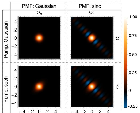
Figure 2. Joint spectral amplitudes in symmetric group velocity matching condition for four different combinations of pump functions and phase-matching function.
