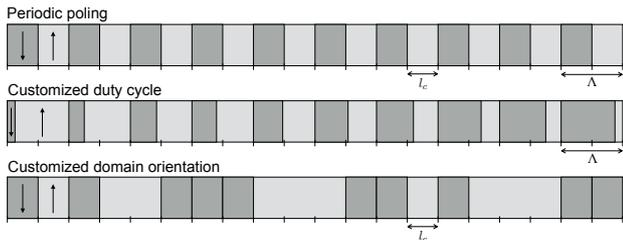
Figure 7. Examples of three poling methods. Periodic poling: periodically alternating fixed-width domains shift the PMF. Customized duty cycle: periodically alternating domains with a customized duty cycle also shift and shape the PMF. Customized domain orientation: fixed-width domains with customized orientations shift and shape the PMF.
