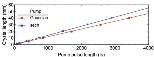
Figure 4. Crystal length as a function of pump pulse duration for periodically poled KTP. Note that the pump duration is defined as the FWHM of the temporal intensity profile of the pulse (that can be measured, e.g., via an autocorrelation measurement). The  $\Delta k$  dependence on the pump, signal and idler frequencies is computed from the Sellmeier equations in [28–30].
