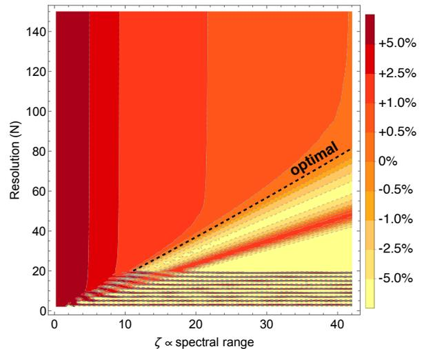
Figure 12. Contour plot of the single-photon purity vs spectral range  $\zeta$  and discretisation resolution  $N$  for a sech pulse group-velocity matched with a sinc-shaped PMF. Different colours correspond to different ranges of purity respect to its most accurate estimate (0.79 – computed with  $\zeta \approx 630$  and  $N = 3000$ ). The black dashed line represents the exact purity value.
