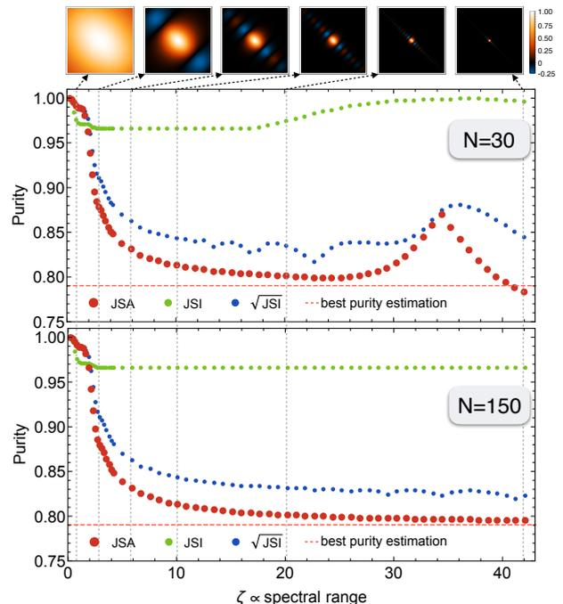
Figure 10. Dependence of the heralded photon spectral purity on the spectral range for two different values of resolution  $N$ . Red points correspond to the inferred purity, while green and blue points correspond to an inferred purity-like parameter computed from Eq. 12 using the JSI or  $\sqrt{\text{JSI}}$ , respectively, in place of the JSA.
