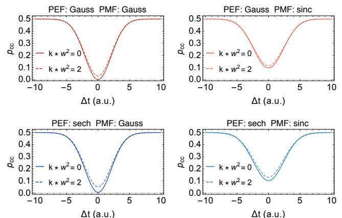
Figure 14. Two-photon interference patterns for four combinations of PEF and PMF shapes in symmetric GVM condition. Both a transform-limited case and a  $kw^2 = 2$  case are considered.
