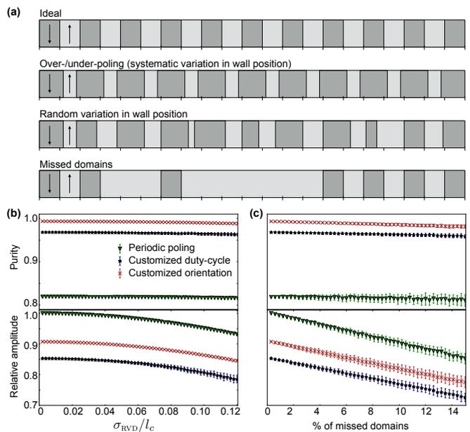
Figure 8. (a) Examples of imperfection profiles on a periodically poled structure. (b) Spectral purity and relative amplitude with random variations in wall positions based on a Gaussian distribution centered around the expected position of each domain, parameterized by the standard deviation  $\sigma_{\text{RVD}}$ . (c) Spectral purity and relative amplitude with randomly chosen missed domains.
