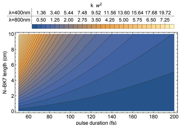
Figure 6.  $kw^2$  in N-BK7 for a sech pulse at different pulse duration and central wavelengths.
