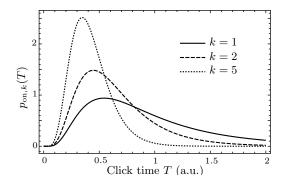
FIG. 2. Firing time probability density function for k=1,2,5 photons arriving simultaneously at time t=0 on a lossless detector with  $\eta=1$  for a log-normal distribution with mean value 1 and standard deviation  $\frac{1}{2}$ .
