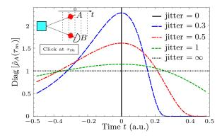
FIG. 4. Density of diagonal elements of the heralded state  $\hat{\rho}_A$  as a function of time for different timing-jitter standard deviations. The source emits pairs of simultaneous photons having a rectangular temporal distribution  $\psi(t)$  centered in 0 and a width equal to 1. Normalization ensures the area under each curve to be 1.
