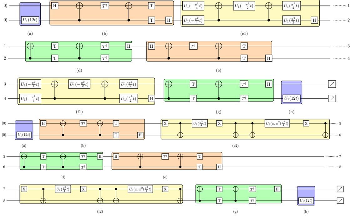
Figure 1: **Quantum circuit for simulating the Klein Gordon equation.** Steps (b) and (d) represent the circuits performing the inverse of the Fourier transform  $F^\dagger$ . Steps (d) and (g) represent the circuit for the Fourier transform  $F$ . Steps (a) and (h) represent the potential term of the Klein Gordon equation. Steps (c1), (c2), (f1), and (f2) are the digital quantum circuit representation for the eigenvalues of the respective eigenfunctions.
