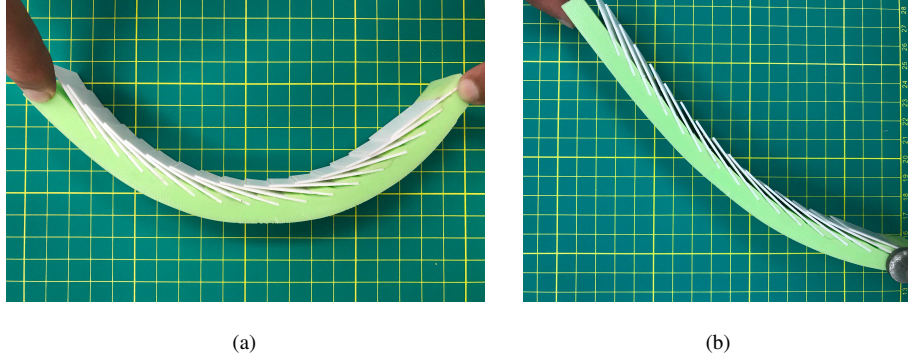
Figure 1: (a) A manual illustration of periodic engagement of scales as the underlying structure bends uniformly. (b) An illustration of non-periodic engagement of scales through the example of a cantilever scaly beam. The substrate and scales were printed using Polylactic Acid (PLA) and Vinylpolysiloxane (VPS), respectively. The dimensions of the fabricated substrate are 200 mm (length) x 25 mm (width) x 5 mm (height) while scale dimensions are 35 mm x 25 mm x 1 mm with inclination angle of 10^\circ . The spacing between scales is 10 mm.
