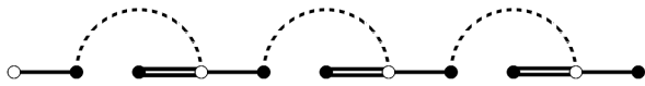
FIG. 3: The spin model generated from x - yx - y bond chain model. Solid lines denote local x -bonds, double solid lines denote local y -bonds, dashed lines denote non-local z -bonds.
