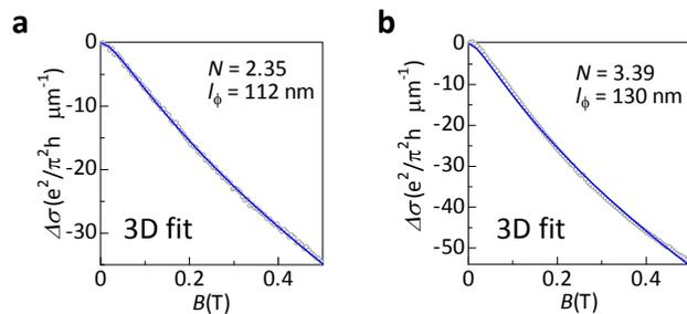
FIG. S2. Low-field MC for quasi-2D films at **a** low ( $n = 1.8 \times 10^{19} \text{cm}^{-3}$ ) and **b** high ( $n = 7.2 \times 10^{19} \text{cm}^{-3}$ ) hole density. Experimental data are shown in open circles. Theoretical fits based on 3D formula are shown in solid lines.
