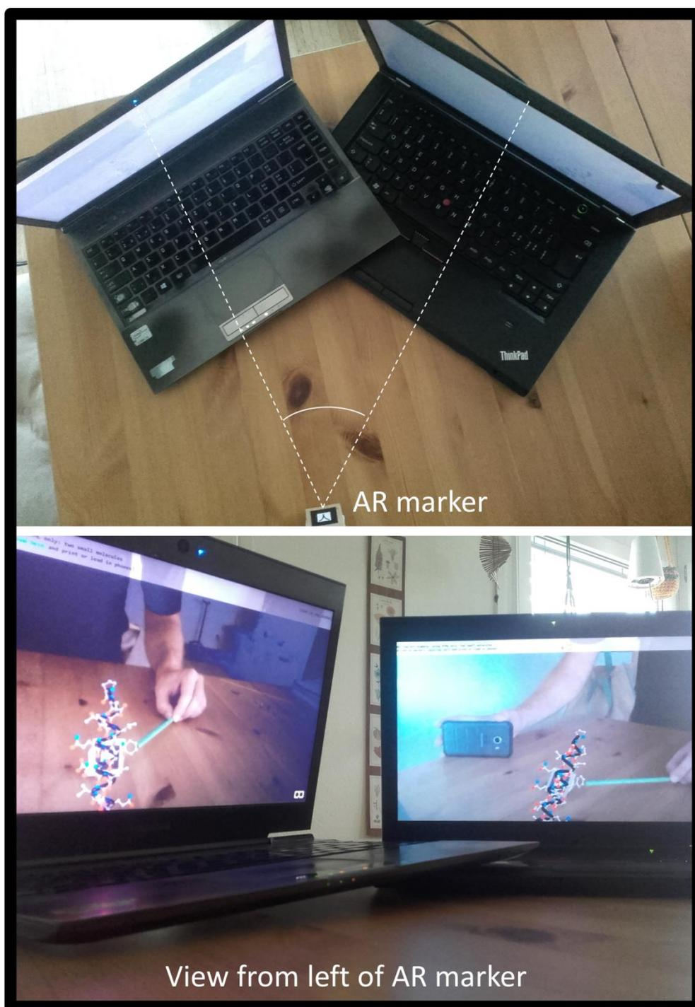
**Figure S4.** The same marker used for augmented reality in two laptops set at around  $30^\circ$  (top). When a user “touches” one residue (a phenylalanine’s aromatic ring in the example) other users see the same from their viewpoints. This is the principle for concurrent, multiuser AR/VR.
