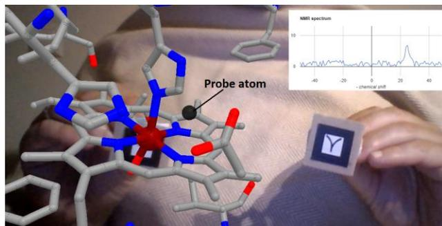
**Figure 2:** The active site of Fe(III) metmyoglobin on the Hiro marker, and a probe hydrogen atom on the Kanji marker. From the polar coordinates of the probe atom in the framework of the heme group, pseudocontact chemical shifts and line broadening are calculated and the corresponding paramagnetic spectrum is simulated, displayed with Google Charts.
