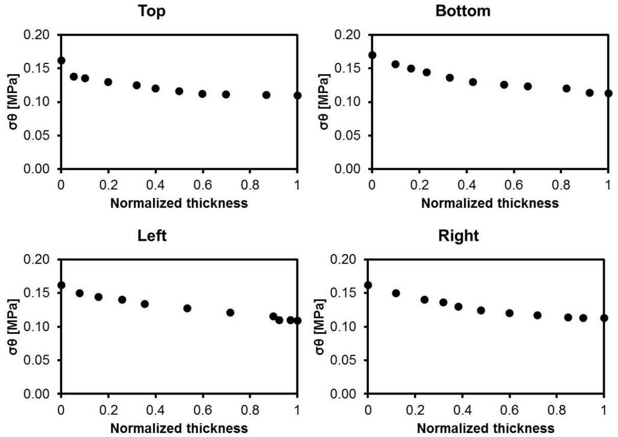
**Figure 7.** Circumferential stress distribution across the vessel wall thickness at different cross-sections.
