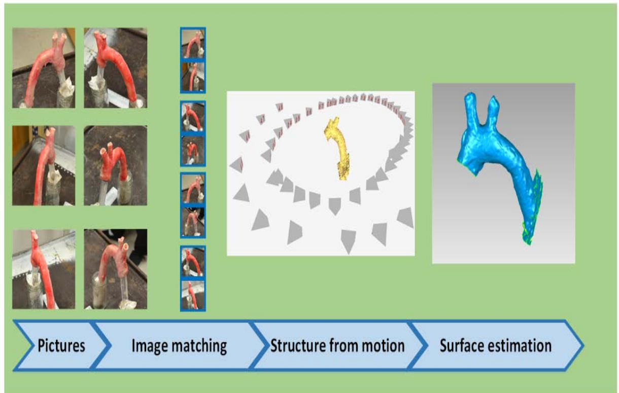
**Figure 1.** Workflow of reconstructing the geometry of aortic arch.
