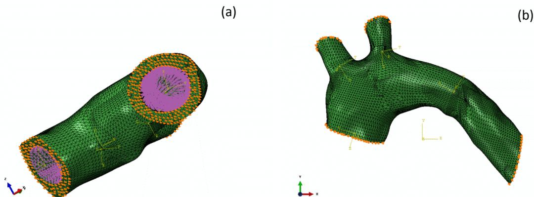
**Figure 3.** Boundary conditions of aortic arch in the modeling. (a) internal pressure; (b) fixed locations during the experiment.
