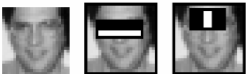
Fig. 1. Left: face detected based on the Haar-like features used by Viola and Jones [4]. Center and right: examples of Haar-like features. Images from the OpenCV documentation [17].
