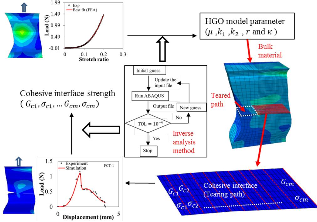
**Fig 4.** Flow chart of the inverse analysis of fibrous cap tearing tests which used to obtain the cohesive interface parameters along the tearing path.
