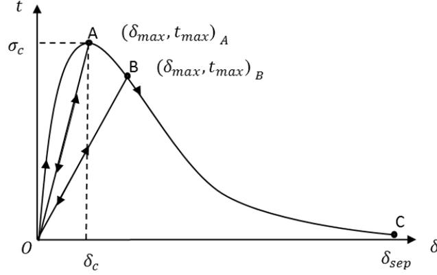
**Fig 2.** Irreversible exponential cohesive model denotes with normalized effective traction and effective displacement.
