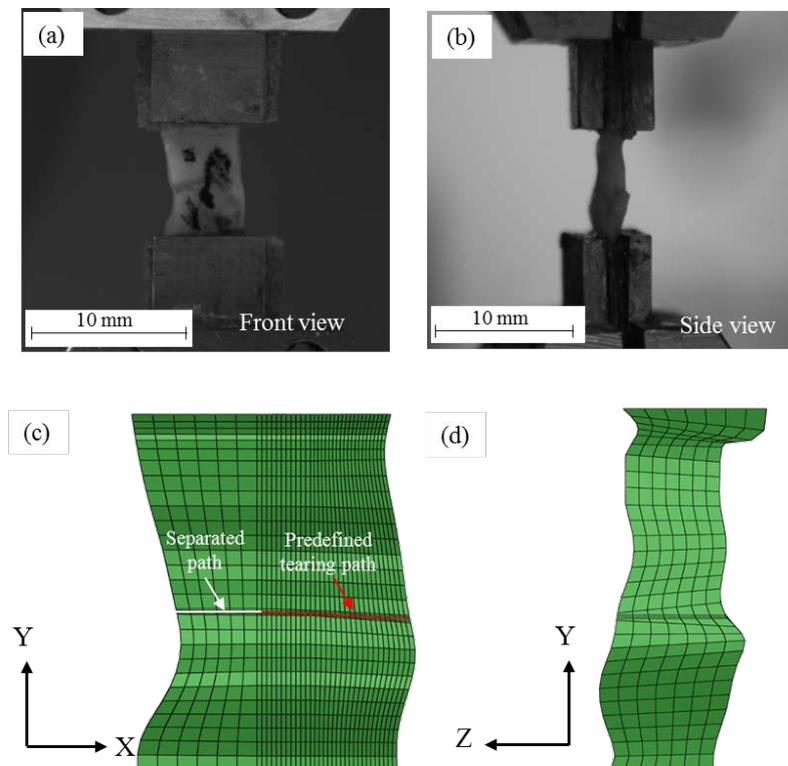
**Fig 3.** Representative experimental images of the fibrous cap tearing specimen: (a) a front view of the specimen; (b) a side view of the specimen; (c) FE model of front view of the specimen, which the white line shows the initial separated path and the red dot line denotes the predefined tearing path that will tear during the experiment; (d) FE model of side view of the specimen.
