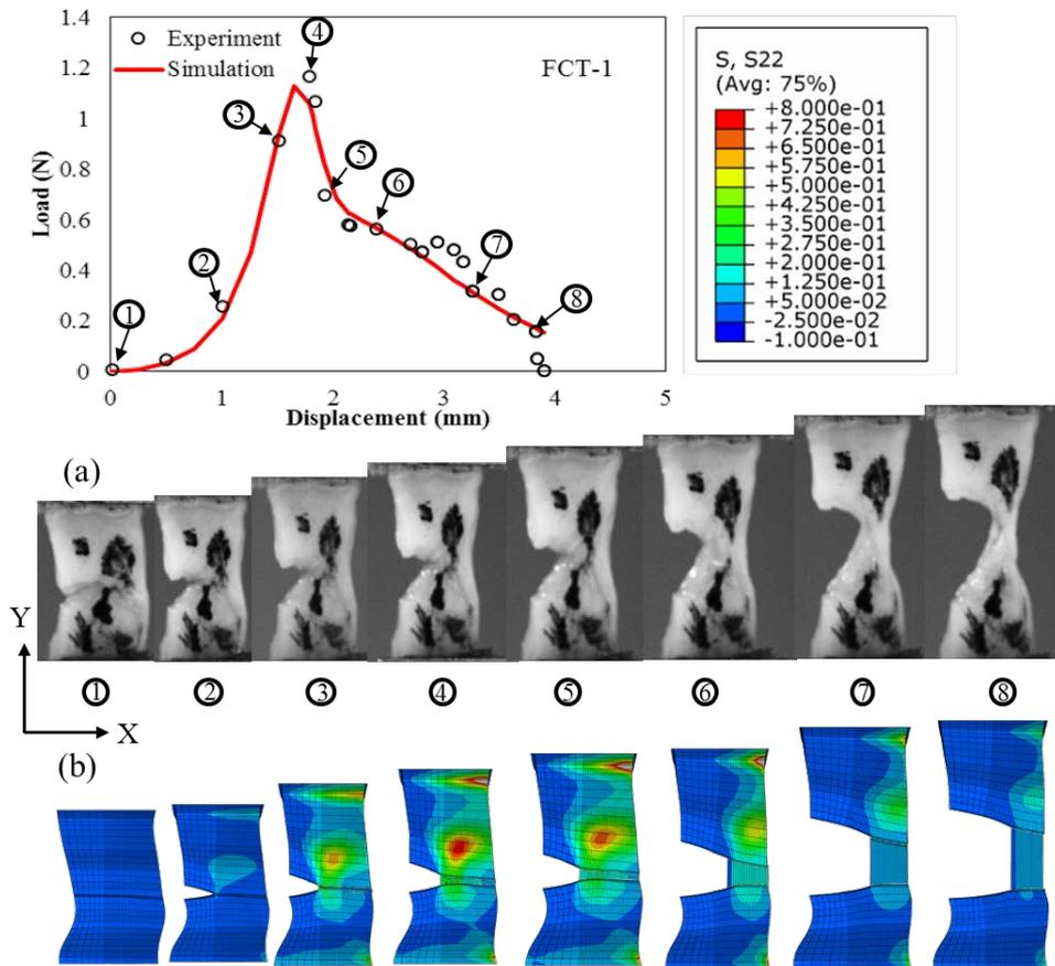
**Fig 7.** Tension stress (S22, along Y direction) contours at eight typical points along the load-displacement curve during tearing process: (a) tension deformation from experiment and (b) simulation prediction.
