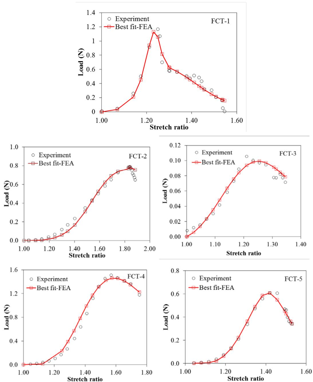
**Fig 5.** The simulation predicted load-displacement curves of loading-tearing cycles are compared with the experimental measured curves.
