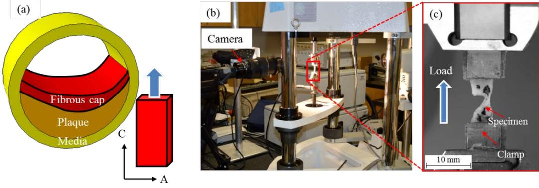
**Fig 1.** Schematic of experimental setup. (a) Schematic of carotid artery plaque specimens obtained from endarterectomies and cut to strips transversely (A: axial direction; C: circumferential direction); (b) Experimental setup of fibrous cap tearing tests; (c) experiment setup (zoomed-in view).
