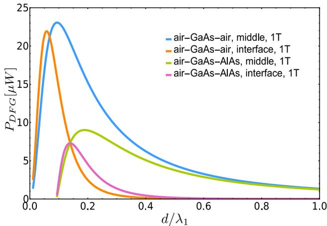
Figure 4. DFG power per  $1 \text{ W}^2$  of the pump power as a function of the waveguide core thickness for the magnetic field strength 1 T. In the legend of the plot “middle” means that graphene is in the middle of the core dielectric  $\epsilon_2$ ; “interface” means that graphene is located at the interface of dielectrics  $\epsilon_2$  and  $\epsilon_3$ . “1T” and “3T” stands for 1 and 3 Tesla magnetic field.
