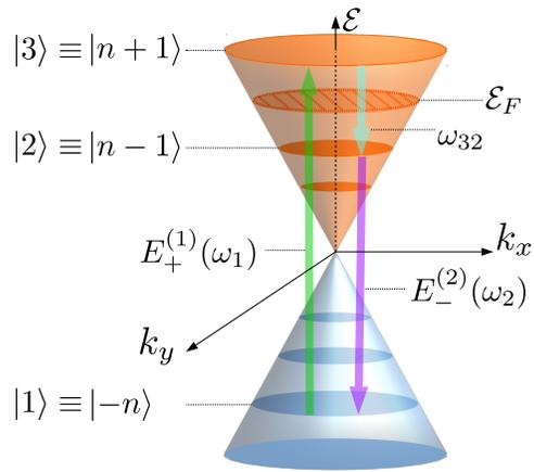
Figure 2. A sketch of Landau levels in graphene (not to scale) superimposed on the Dirac cone and the resonant DFG scheme. The pump fields  $E_{\pm}$  are coupled to electric-dipole allowed Landau level transitions. The difference frequency field is resonant to a dipole-forbidden transition.
