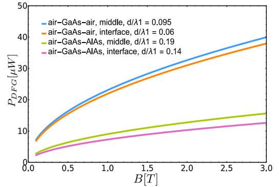
Figure 6. The DFG power per  $1 \text{ W}^2$  as a function of the magnetic field for several waveguide structures and geometries. In the legend of the plot “middle” means that graphene is in the middle of the core dielectric  $\epsilon_2$ ; “interface” means that graphene is located at the interface of dielectrics  $\epsilon_2$  and  $\epsilon_3$ .
