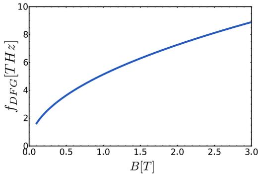
Figure 3. The DFG frequency resonant to the transition between Landau-level numbers 2 and 4 as a function of the magnetic field strength.
