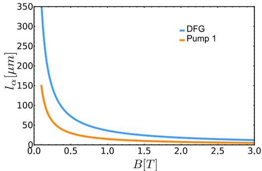
Figure 7. Absorption length for pump field intensity and DFG plasmon-polaritons as a function of the magnetic field for a symmetric GaAs waveguide with graphene at the interface. The core thickness is  $0.06\lambda_1$ .
