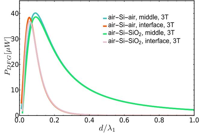
Figure 5. DFG power per  $1 \text{ W}^2$  as a function of core thickness for the magnetic field strength 3 T. A higher magnetic field is chosen to avoid THz absorption in Si.
