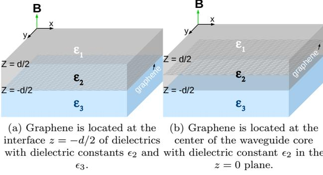
Figure 1. A sketch of integrated waveguide geometries.
