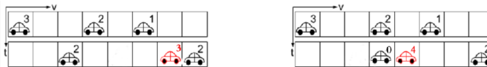
Figure 1. (Color online) Schematic graph of updating and moving in the NSOS model. The numbers in the sites represent the velocities after moving. The red cars are overtaking vehicles (left). The second car is an overtaking vehicle, it has tried to overtake the preceding one but failed (right). The first car is an overtaking vehicle, it has successfully overtook the preceding one.
