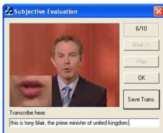
Figure 3.7: A screenshot of the evaluation program used for Lip Assistant, with the synthesised mouth sequence superimposed over the video of a speaker. Image from [140].
