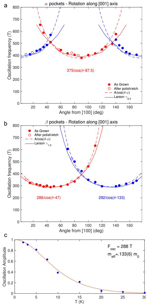
FIG. 3: (a) Angular dependence of the dHvA oscillation frequency for the  $\alpha$  pocket. (b) Angular dependence of the dHvA oscillation frequency for the  $\beta$  pocket. (c) Thermal damping of the  $\beta$  oscillation at  $45^\circ$  from [100].
