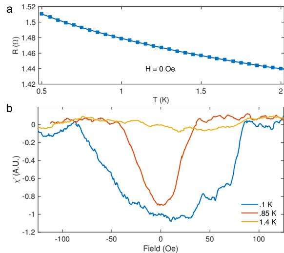
FIG. 4: (a) Resistance versus temperature in zero applied field for a  $\text{SmB}_6$  crystal with a subsurface Aluminum inclusion. (b) AC Susceptibility measurement of  $\text{SmB}_6$  crystal near zero field.
