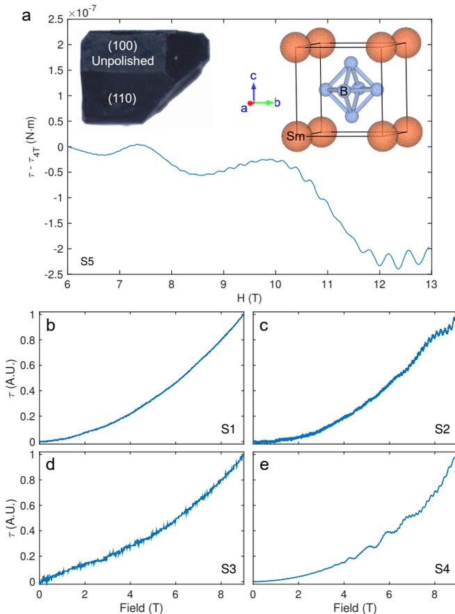
FIG. 1: (a) Torque magnetization as a function of magnetic field of a representative  $\text{SmB}_6$  single crystal (s5). To focus on the oscillations, the value of the torque at 4 T was subtracted from the data. The inset shows a picture of the as-grown sample along with its cubic crystal structure. (b-e) A survey of several  $\text{SmB}_6$  crystals that were checked for quantum oscillations using torque magnetometry. Only samples s2 and s4 showed oscillations.
