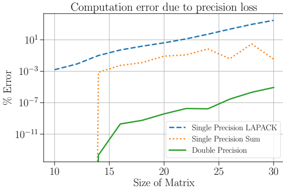
Figure 4: Comparison of Hafnian computation error due to using single precision for LAPACK and performing the summation. Clearly, the error due to low precision LAPACK dominates over the summation error. This indicates that the errors can further be controlled by employing quad precision LAPACK and summation.
