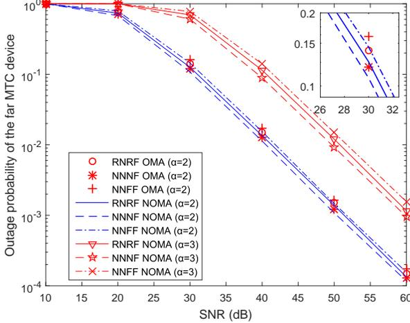
Figure 4. Outage probability of the far MTC device vs. SNR for different values of the path loss exponent.
