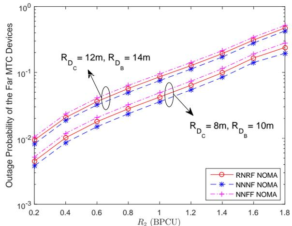
Figure 8. The outage probability of the far MTC device vs.  $R_2$  with different  $R_{D_C}$  and  $R_{D_B}$  in the three pairing schemes.
