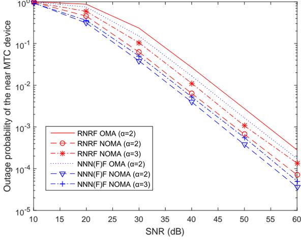
Figure 3. Outage probability of the near MTC device vs. SNR for different values of the path loss exponent.
