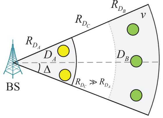
Figure 1. The proposed mmWave-NOMA downlink transmission scheme in cellular M2M communications for IoT, which include a BS and two groups of MTC devices,  $A = \{A_i\}$  and  $B = \{B_j\}$  located in the regions  $D_A$  and  $D_B$ , respectively, which have a central angle of  $2\Delta$ . Distributions of the near MTC device (yellow circles) and the far MTC device (green circles) follow HPPPs. The MTC devices located in  $D_A$  and  $D_B$  will be scheduled.
