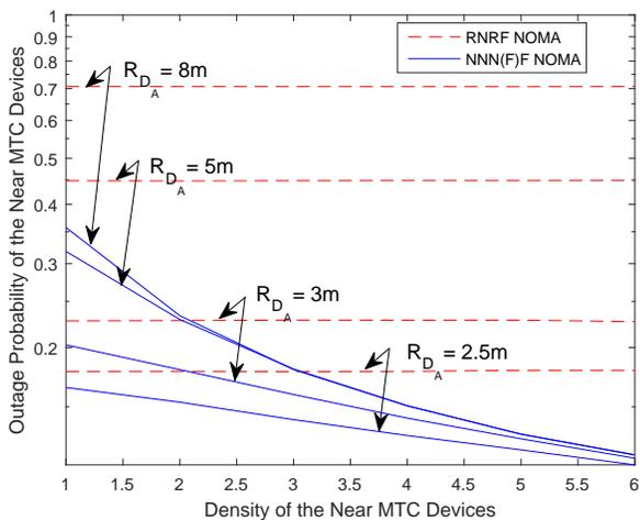
Figure 7. The outage probability of the near MTC device vs. density of the near MTC device with different  $R_{D_A}$ , where  $R_1 = 2.5$  BPCU,  $R_2 = 1$  BPCU,  $R_{D_C} = 12$ , and  $R_{D_B} = 14$ .
