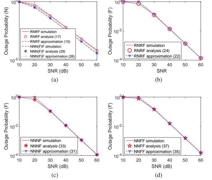
Figure 2. Outage probability of MTC devices vs. SNR. (a) the near MTC device in the three MTC device pairing schemes; (b) the far MTC device in RNRF; (c) the far MTC device in NNNF; (d) the far MTC device in NNFF.
