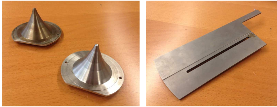
Figure 1: Left: old and new flattening filters. Right: Leaf from the MLC
