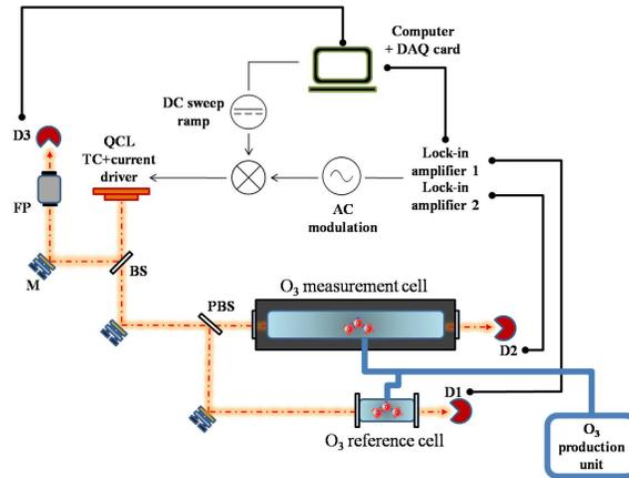
Figure 1: Schematic of the experimental setup: QCL, distributed feedback quantum cascade laser; BS, beam splitter; PBS, polarizing beam splitter; FP, Fabry-Pérot étalon; D, detector; DAQ card, data acquisition card; TC, temperature controller.
