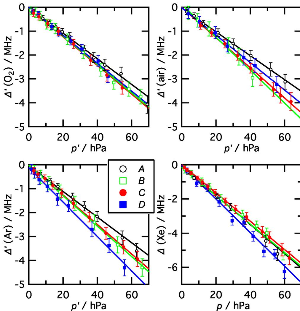
Figure 4: Pressure shift of  $A - D$  lines for four different perturber gases:  $O_2$ , air, Xe, and Ar. Error bars indicate standard uncertainties (at coverage of  $k = 1$ ) in the measured quantities.
