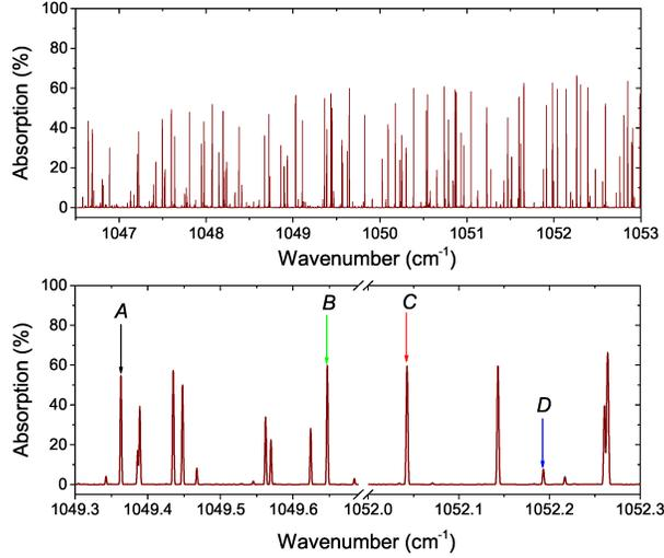
Figure 3: Upper panel: ozone absorption in the tuning range of our QCL. The absorption signal is calculated using the HITRAN2016 data. Lower panel: Measured absorption spectrum giving a zoom on the two spectral windows ( $1049.3 - 1049.6 \text{ cm}^{-1}$  and  $1052 - 1052.3 \text{ cm}^{-1}$ ), where the four selected lines are situated.
